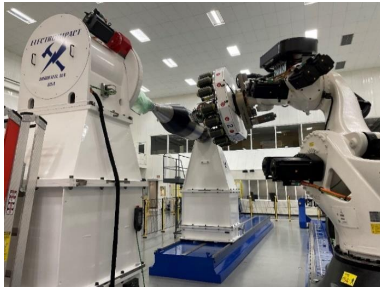
Figure 4. Test article being manufacture with MSFC's automated fiber placement robot.
