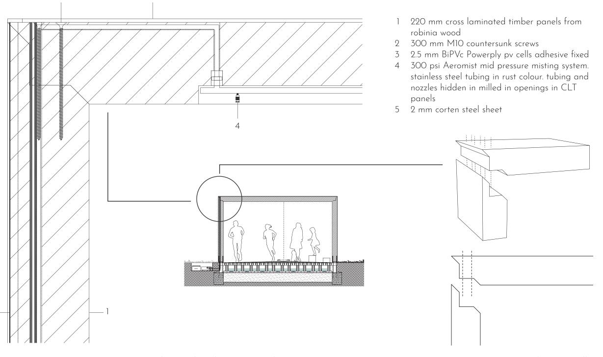
corner connection of portal with integrated water spray | 1:5 corner connection schematically
