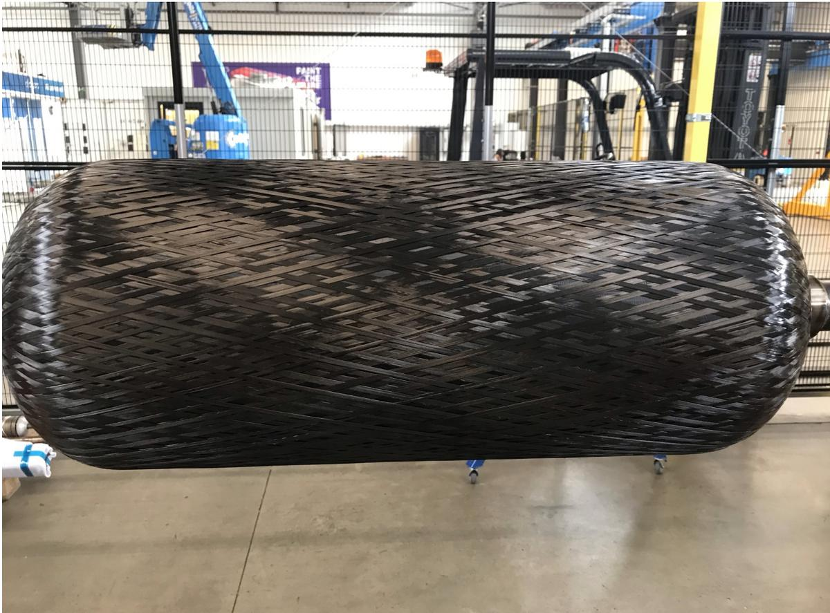
**Figure C.4:** Voids in the winding pattern, caused by folded tape
