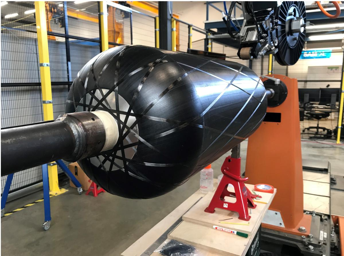
Figure 2.8: AFP robot head used for filament winding of a CPV at the samXL facility
