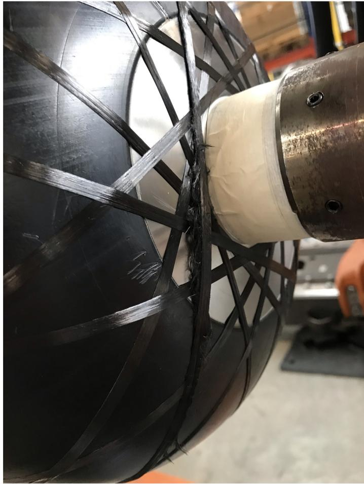
**Figure C.3:** Loose fibres positioned on the mandrel
