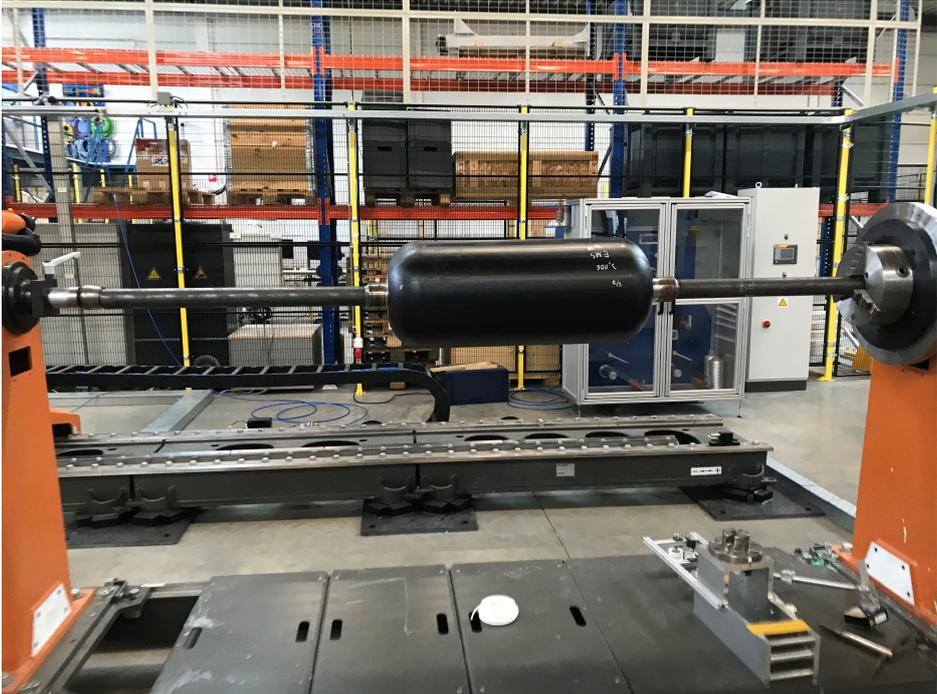
Figure 5.2: Mandrel fitted in the fixture at the samXL facility
