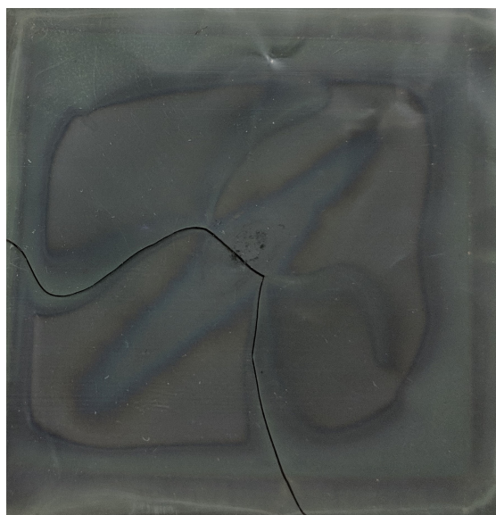
Figure 5.1: Marks on the fuel side of the ReSOC which indicate a flow pattern.
