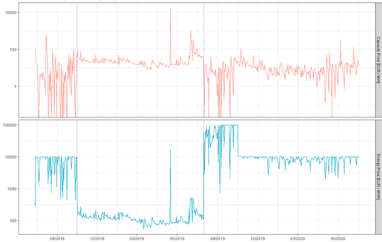
Fig. 1. The evolution of marginal prices for positive aFRR, balancing capacity (top) and balancing energy (bottom) in Germany from end of 2018 to mid-2020. The period during which ‘mixed price calculation’ was in force is marked with dashed lines. Please note that the logarithmic scale is used.
