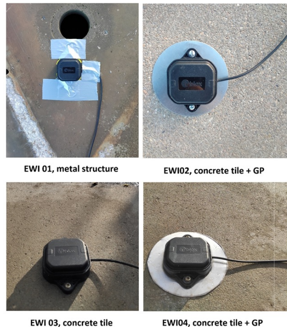
Figure 6. Emplacement of each antenna (surface type and GP or no GP). Metal disc as ground plane (GP). Each picture is pointing to the South.
