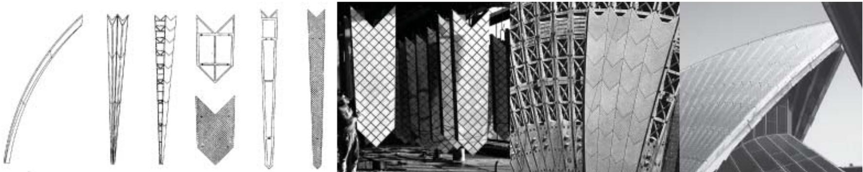
Fig. 2.4. Precast spherical element principles of the tiles and with the glass enclosures on the right<sup>11</sup>
