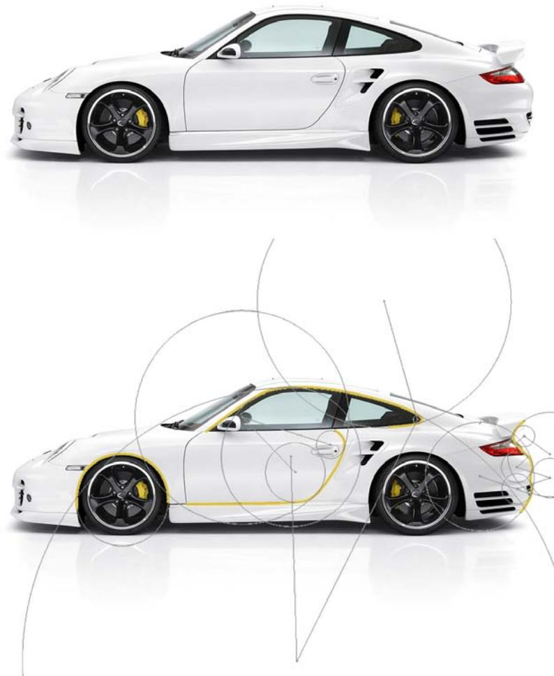
Fig. 2.18. Approximation of some freeform curves on a Porsche 911 Turbo [<http://www.dieselstation.com>, January 2010]. It must be noted that the complexity of the geometric description of curves and surfaces, both in modelling as in fabrication, in the automotive industry is more advanced than in the building industry, partly because of the possibilities of mass-production, making this example a little presumptuous
