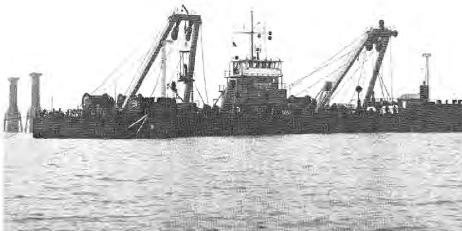
Fig. 1 DOS-pontoon with two cone penetration testing/boring rigs.
