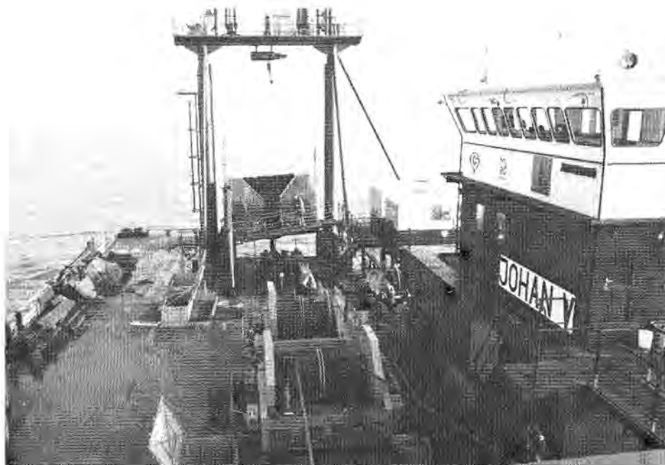
Fig. 2 View of the cone penetration testing and boring equipment.
