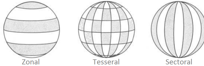
Figure 3.11: Zonal, tesseral and sectorial spherical harmonics [Pisacane, 2005]
