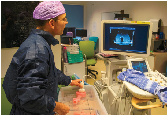
(a) The IR performs the intrahepatic puncture step with the steerable stylet in the liver model. The image of the ultrasound probe is visible on the monitor.
