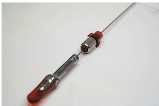
(c) By loosening the threaded lock and turning the handle a quarter against the front part, the two parts can be disconnected.
