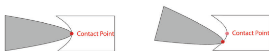
(a) Two halves in a parallel state. (b) Two halves after a rotational movement.
