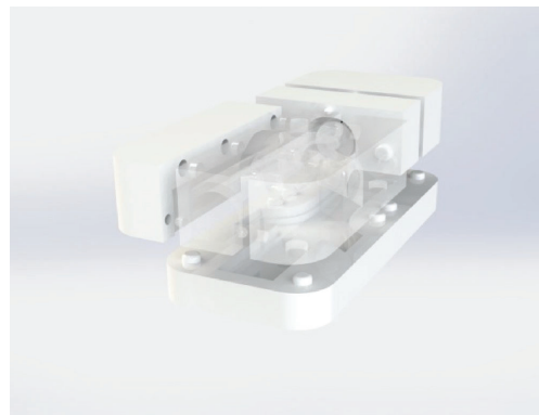
(b) Mold to produce a PVA sample of the jugular vein, superior and inferior vena cava.
