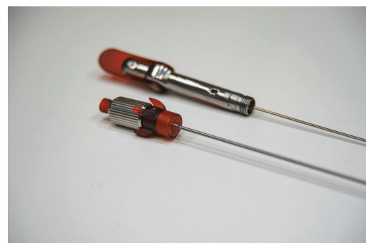
(d) The front part of the handle is disconnected. The tip of the stylet is not able to steer since the steering mechanism does not have the fixation of the rigid cannula.
