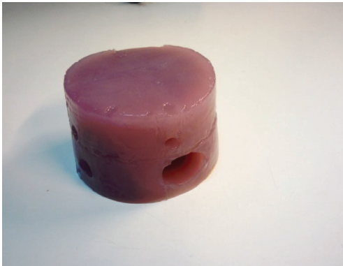
(c) The liver part of the test model, made of the PVA mixture with some red pigment.
