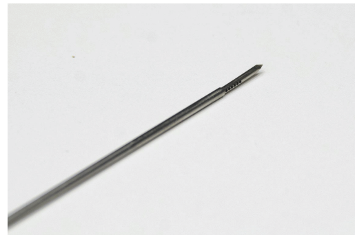
(b) A close up of the tip of the TIPS stylet with the rigid cannula around.
