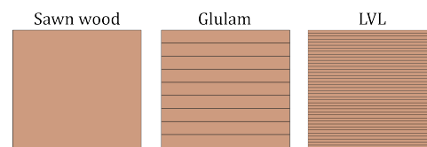
Figure 5.2: Build-up of a beam of sawn wood, glulam or LVL
