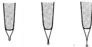
**Figure A.4:** Microdripping mode; different stages of drop formation. Taken from [7].
