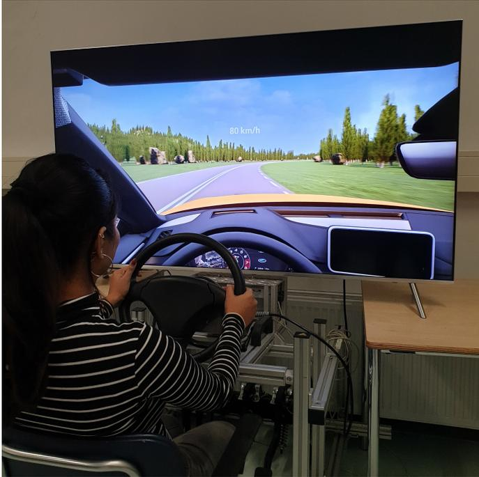
Fig. 3. Participant driving in the fixed-base driving simulator.
