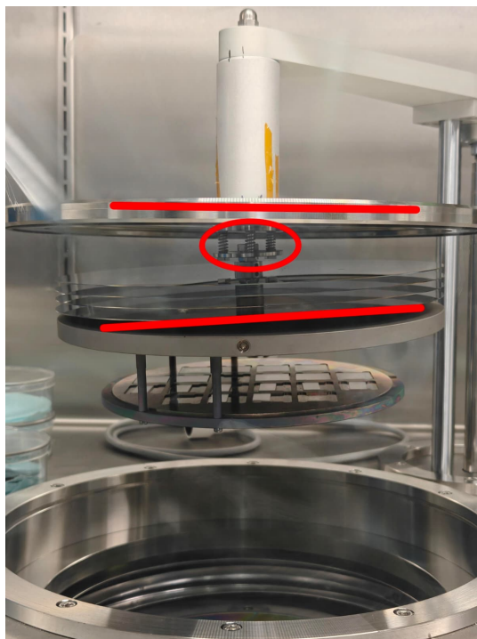
Figure 5.1: Tilted sample holder rack due to the screws loosening over time marked in the red circle.
