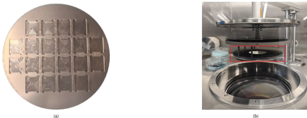
Figure 3.1: The (a) 20-slot substrate holder used to accommodate up to 20 substrates with dimensions of 2.5 x 2.5 cm and (b) the Picosun R200 ALD reactor with the lid open, with the red rectangle indicating the location where the substrate holder lays.
