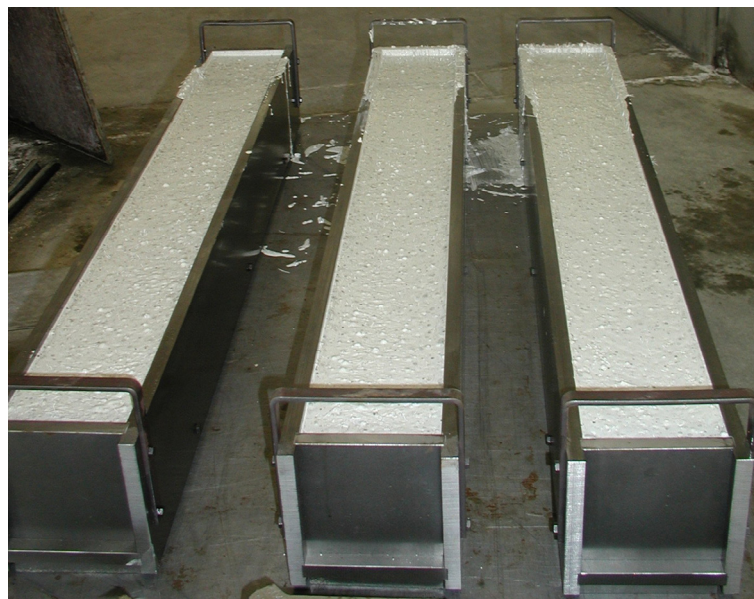
Figure 3.1: Moulds for the four point bending tests filled with BSI/CERACEM.
