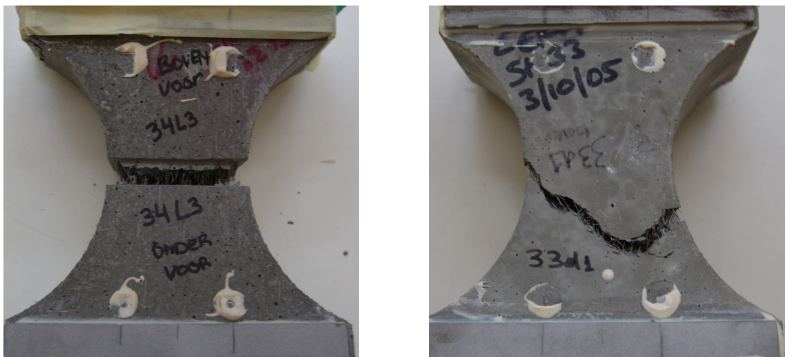
Figure 4.27: The main crack in a notched and an un-notched specimen.
