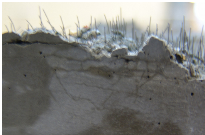
Figure 4.28: Crack surface of an un-notched tensile specimen; visible are pulled-out fibres and fine distributed cracks close to the main crack surface
