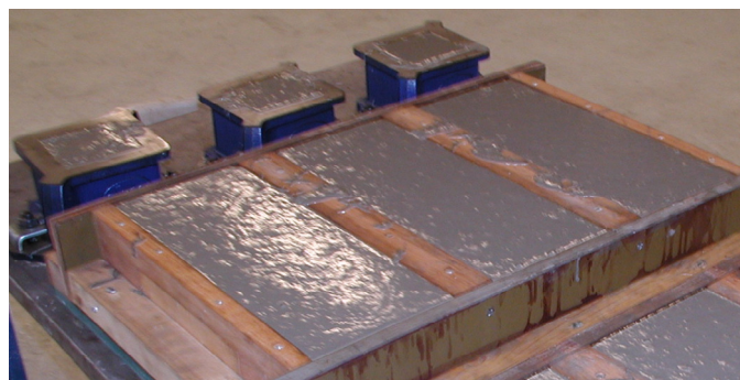
Figure 3.2: Timber moulds for the dogbone tensile HSFRC specimens.
