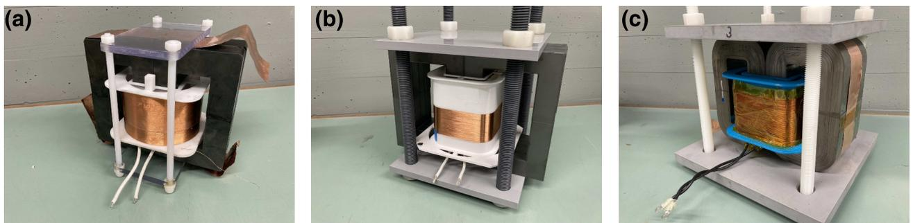
FIGURE 9 Photographs of three transformer designs. (a) Transformer PT1:  $A_e = 3360$  mm<sup>2</sup>,  $m = 6.0$  kg [9]. (b) Transformer PT2:  $A_e = 4480$  mm<sup>2</sup>,  $m = 10.4$  kg [11]. (c) Transformer PT3:  $A_e = 4600$  mm<sup>2</sup>,  $m = 14.2$  kg.
