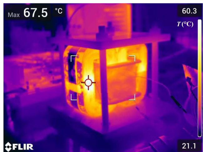
**FIGURE 13** Thermal image of HF transformer 3 using an amorphous cut core at  $f_s = 50$  kHz,  $U_p = 200$  V, and  $U_{DUT} = 4$  kV<sub>pk</sub>. Estimated core losses  $P_c = 280$  W. The region around the cut is approx. 30°C hotter than the rest of the core.
