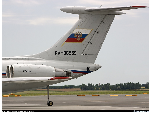
Figure 6.11: Tail wheel on the Ilyushin IL-62M, to prevent tip-over during ground handling [76]
