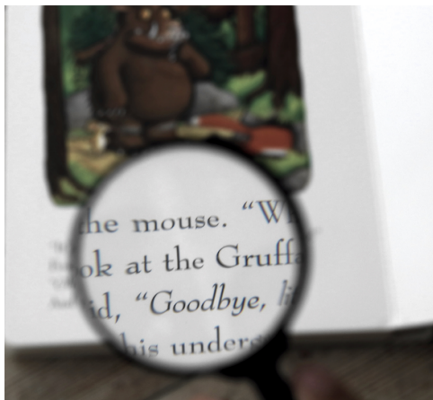
Figure 3.8: Example of a positive lens used as a magnifying glass (picture taken by A.J.L. Adam / CC-BY-SA 4.0).
