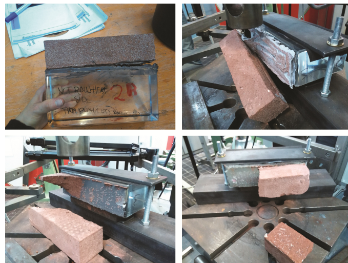
Figure 3. Failure mode in shear of the different types of adhesives. Top Left: Tec7 Brown . Top Right: Sabatack 780 . Bottom Left: Araldite 2013 . Bottom Right: MD-MS Polymer .
