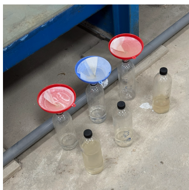
Figure D.8: Suspended Sediment Concentration Setup in progress (Authors, 2025)
