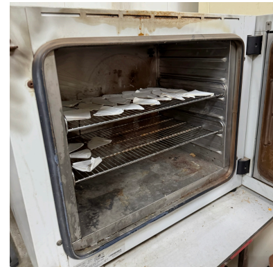
Figure D.12: SSC Filters in the Oven (Authors, 2025)
