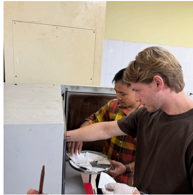
Figure D.11: Putting the SSC Filters in the Oven (Authors, 2025)
