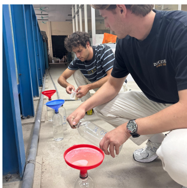
Figure D.7: Preparing the SSC filters (Authors, 2025)
