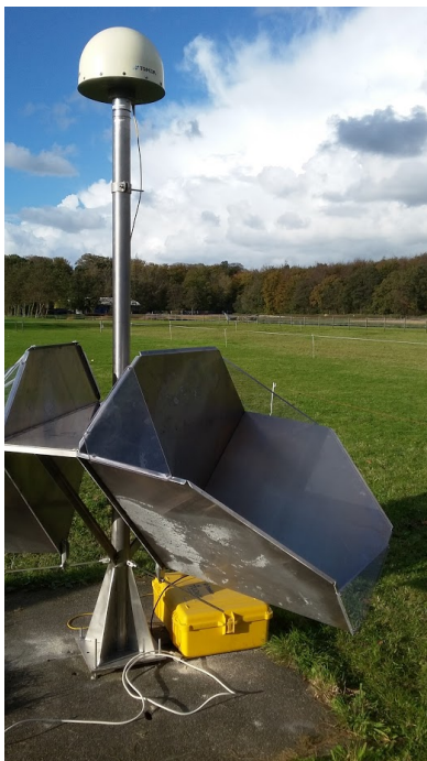
Figure 4.13: Prototype DBF90X-GNSS: Descending reflector.
