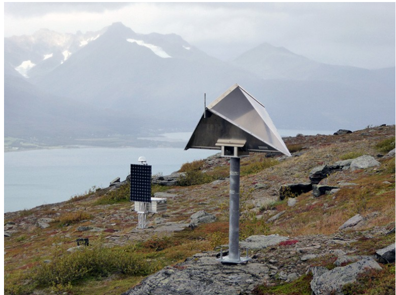
Figure 2.24: ] Co-located corner reflector system (front) in close proximity of a continuous GNSS station (back) in Norway by the Geological survey of Norway (NGU). (Photo: ©NGU)
