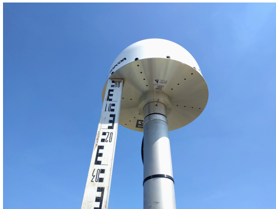
Figure 6.12: GNSS antenna with the levelling rod below.
