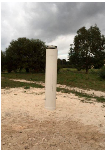
Figure 2.18: Continuous GNSS antenna placed on concrete monument used by Parker et al. in [25].
