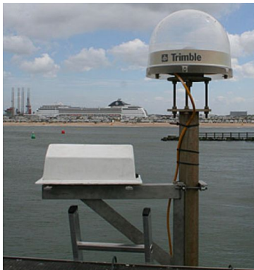
Figure 2.23: Monitoring set up of a continuous GNSS antenna equipped with a transponder by Mahapatra et al. in [7].
