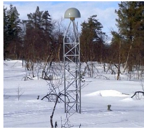
Figure 2.11: Example of a EUREF GNSS station. This station is located in Hetta, Finland. (Photo: ©Royal observatory of Belgium)
