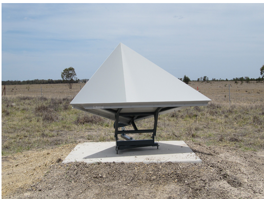
Figure 2.12: Example of a radar reflector. This one is located in Surat Basin, Queensland, AU. (Photo: ©Geoscience Australia)
