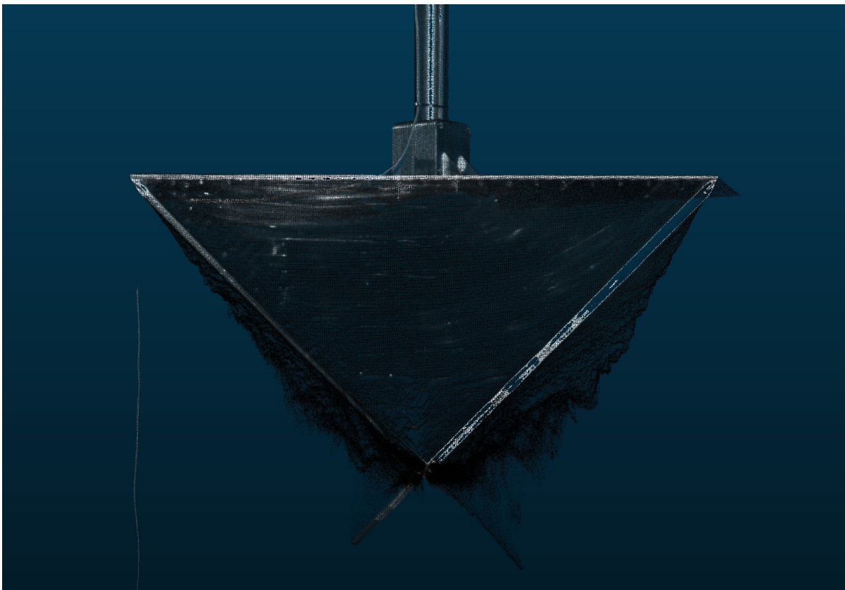
Figure B.1: Frontal view of a reflector on the mock-up. False reflections are present outside the geometry of the corner reflector. They are caused by the mirroring properties of the aluminium side panels. The LiDAR instrument assumes a straight Line-of-Sight while in fact the signal has reflected on the way back and forth.
