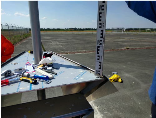
Figure 6.14: Proper way to place the rod on one of the bolts.
