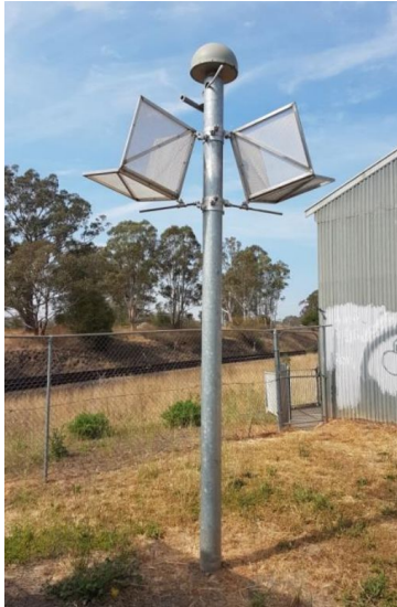
Figure 2.21: Experimental set up of a continuous GNSS antenna equipped with CRs by Fuhrmann et al. in [8].
