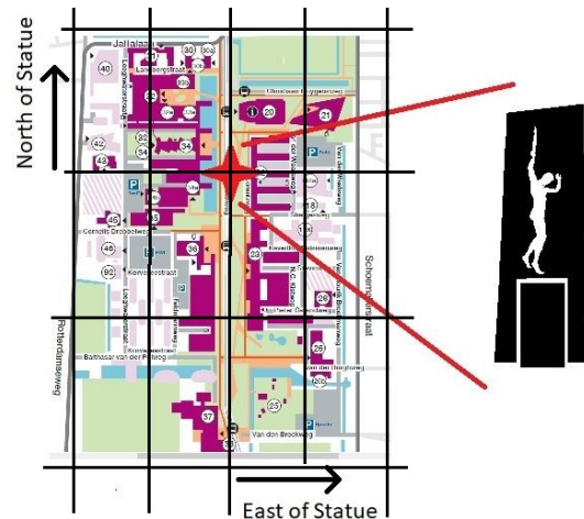
Figure 2.2: Orthogonogal grid on campus representing the campus-datum example sketched in the text. The red cross represents the location of the Prometheus statue, which is the origin of this hypothetical grid.
