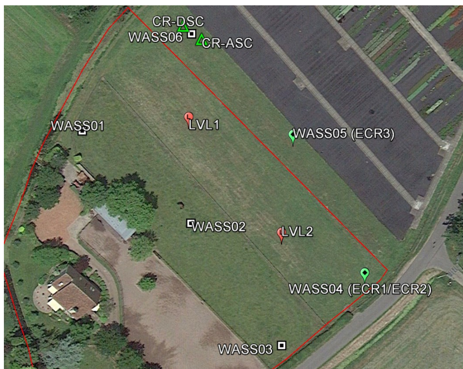
Figure 5.4: Google Earth image of the Wassenaar test site, showing the location of the reference Corner Reflectors CR-DSC for descending tracks and CR-ASC for ascending tracks near concrete slab WASS06. The concrete slabs WASS01 and WASS03 have been used for testing the IGRSs. LVL1 and LVL2 are the locations from where regular levelling is carried out. The electronic corner reflectors (ECR#) are installed for another project, but can be used as (alternative) reference in this project. [46]
