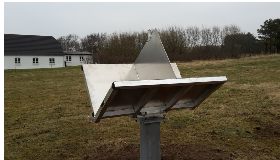
Figure 2.26: Collocated corner reflector system including levelling benchmarks (side) and GNSS mount (top). In use by the Agency for Data Supply and Efficiency in Sweden (SDFE). Designed by: SDFE, Lemvig Water & Wastewater and DTU Space. (Photo: ©SDFE)
