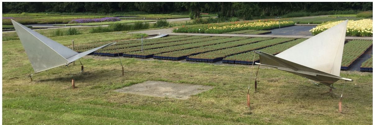
Figure 5.10: The two reference corner reflectors. The corner reflector in the left is used for descending tracks, the corner reflector on the right for ascending tracks. the kind of concrete slab that is used to mount reflectors at the test site can be seen in the middle.
