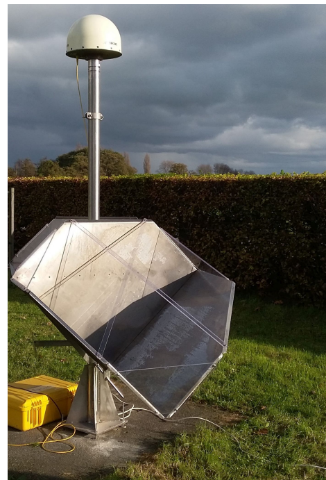
Figure 4.14: Prototype DBF90X-GNSS: Ascending reflector.
