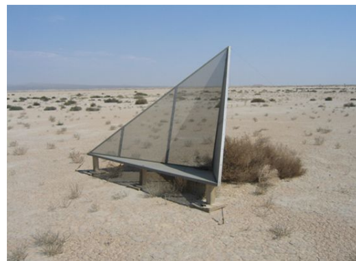
Figure 2.13: Example of a radar reflector. This one is located in Rosamond Dry Lake Bed, California, USA. (Photo: ©Jet Propulsion Laboratory)
