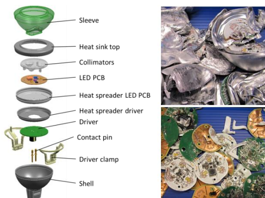
Figure 7 Redesign of MR16 LED lamp made of stacked parts of deep-drawn aluminum. Recycling results are shown for the lamp without and with (sand) potting.
