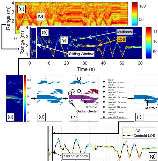
Fig. 2. Flowgraph providing insights from Fig. 1(a). (a) Initial RT map with LOS and multipath components, (b) selection of the  $k$ -strongest range bins, (c)–(f) clustering steps to delineate the LOS cluster from noise and multipath, and (g) refined RT map featuring the LOS signal and its centroid.
