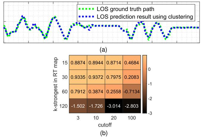
Fig. 4. Results of the clustering algorithm's parameter optimization. (a) Identified LOS path using the optimized parameters  $k$ -strongest = 30 and cutoff = 10, yielding an  $R^2$ -score of 93.72%. (b)  $R^2$ -scores obtained through a brute-force evaluation method.
