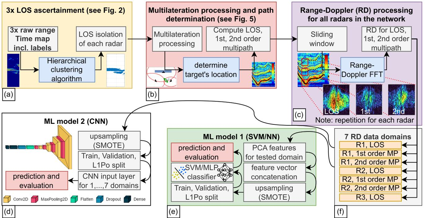
Fig. 1. Proposed processing pipeline for multipath exploitation in human activity classification (HAR) with two classifier pipelines tested. The blocks of (a) *LOS ascertainment*, and (b) *multilateration processing and path determination* are explained in more detail in Figs. 2 and 6, respectively, followed by the pipeline's blocks, (c) range-Doppler extraction, (f) data domain overview, (e) machine learning (ML) model 1 and (d) ML model 2.
