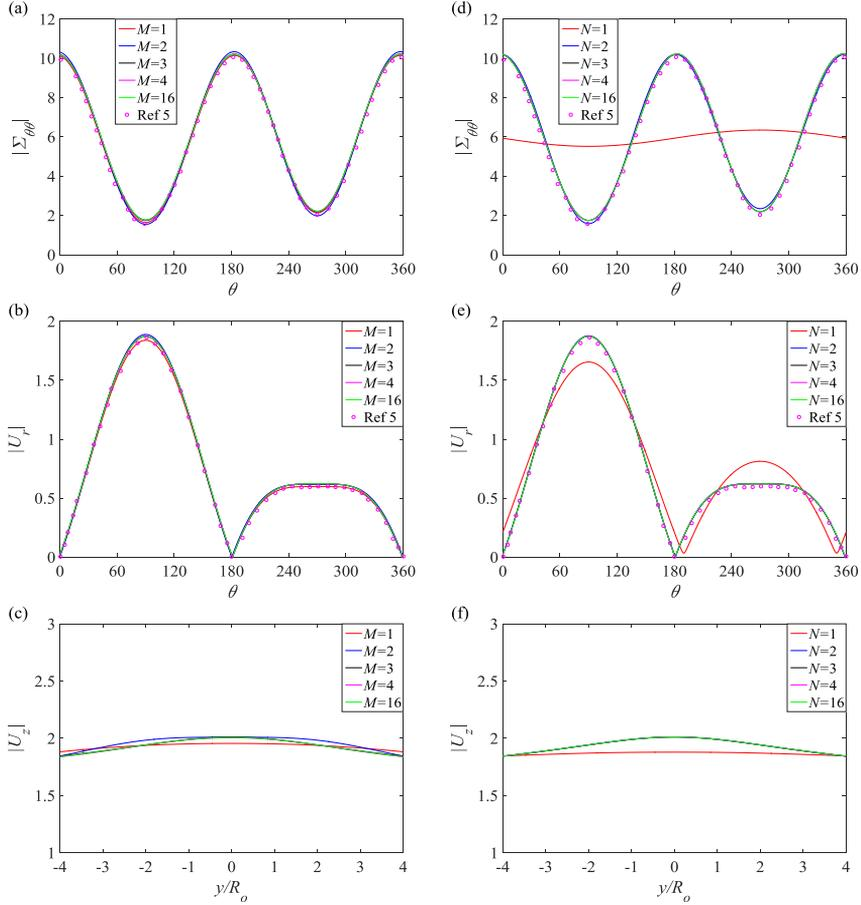
**Fig. 4** Three-dimensional case convergence tests and validations (a-c) Modes  $M$  for the secondary reflected waves with  $N = 3$ ; (d-e) Modes  $N$  for the directly scattered waves by the cavity with  $M = 3$ ; (a), (d) Normalized hoop stress at  $r = R_C$ ; (b), (e) Normalized radial displacement at  $r = R_O$ ; (c), (f) Normalized vertical displacement at  $z = 0$ ;  $\theta_v = 30$ ,  $\theta_h = 0$ ,  $h = 5R_i = 4.545R_o$ ,  $\varpi = 0.105$
