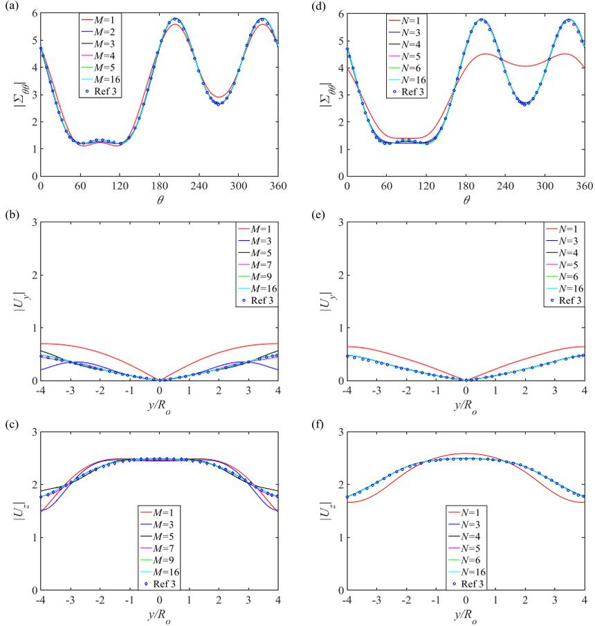
**Fig. 3** Two-dimensional case convergence tests and validations: (a-c) Modes  $M$  for the secondary reflected waves with  $N = 6$ ; (d-f) Modes  $N$  for the directly scattered waves by the cavity with  $M = 9$ ; (a), (d) Normalized hoop stress at  $r = R_o$ ; (b), (e) Normalized horizontal displacement at  $z = 0$ ; (c), (f) Normalized vertical displacement at  $z = 0$ ;  $\theta_v = 0$ ,  $\theta_h = 90$ ,  $h / R_o = 5$ ,  $\varpi = 0.5$
