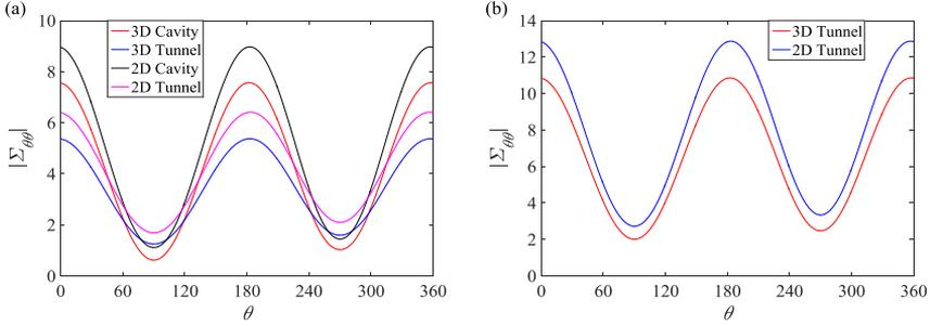
**Fig. 5** (a) Normalized hoop stress at  $r = R_o$  ; (b) Normalized hoop stress at  $r = R_c$  ;
