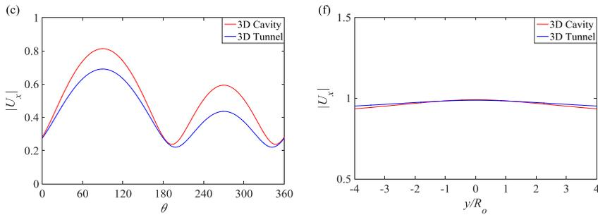
**Fig. 6** (a-c) Normalized displacements at  $r = R_o$ ; (d-f) Normalized displacements at  $z = 0$ ;  $N = M = 4$ ,  $h = 5R_o$ ,  $\varpi = 0.105$ , 2D case ( $\theta_v = 0$ ,  $\theta_h = 90$ ), 3D case ( $\theta_v = 30$ ,  $\theta_h = 0$ )
