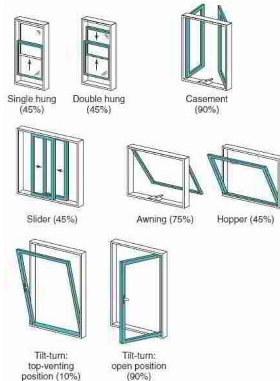
Figure 3.5. Operable window areas for natural ventilation for different window types [27]
