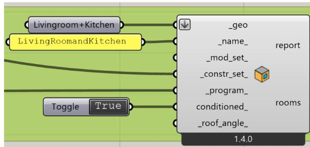
Figure 4.5. Script showing how rooms are defined in honeybee. All the components for the construction set and program types are connected to the room.
