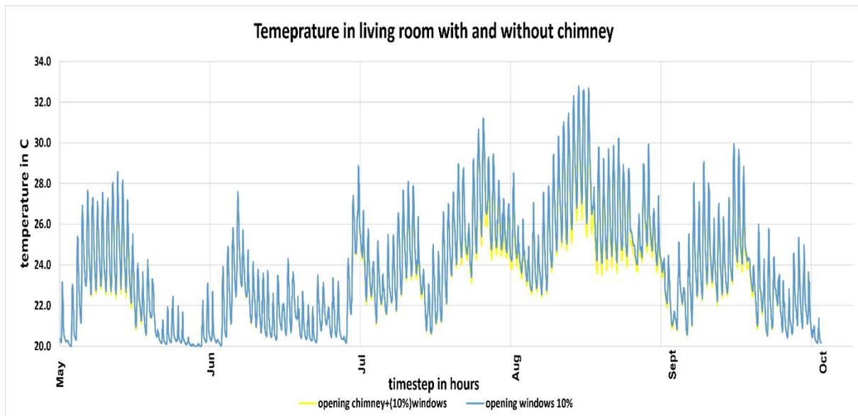
Figure 6.8. Temperature in the living room when the chimney of 0.2m by 0.2m in size is used.
