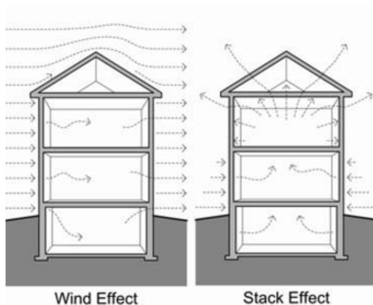
Figure 2.1. Picture showing airflow through buildings due to wind and stack [9]
