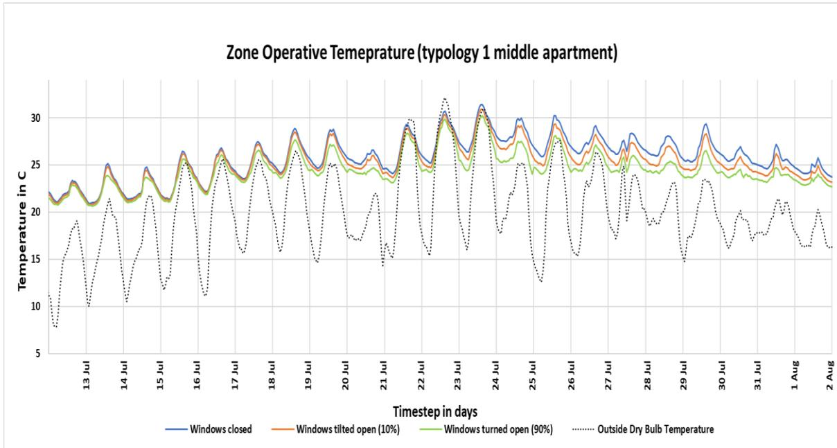
Figure 6.2. Zone operative temperature of center apartment for three cases. The blue line represents the zone temperature when the windows are closed. The orange line represents the zone temperature when the windows are opened in the tilt position where only 10% of the glazed surface is open. The green line represents the window open in turned position where 90% of the glazed area is available for ventilation. (full graph in Appendix D)
