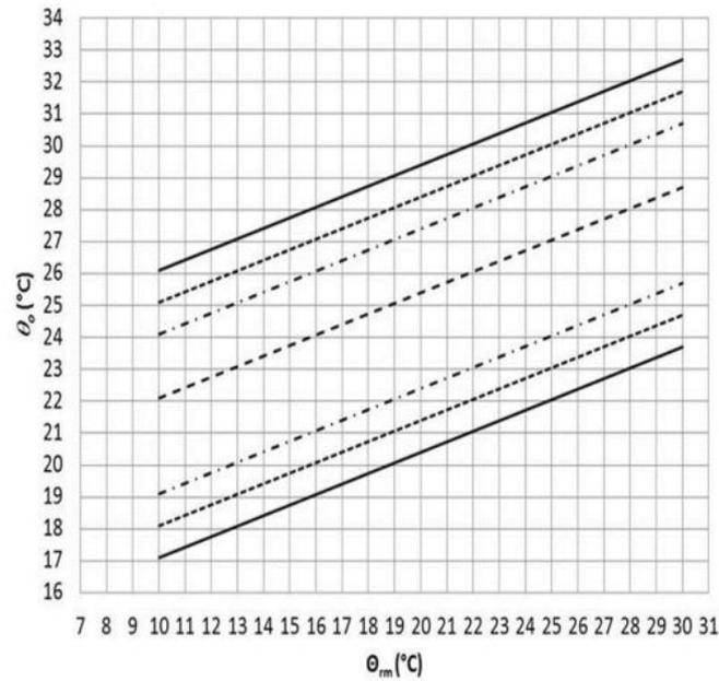
Figure 2.3. Acceptable operative temperature ranges for buildings without mechanical cooling systems [16]
