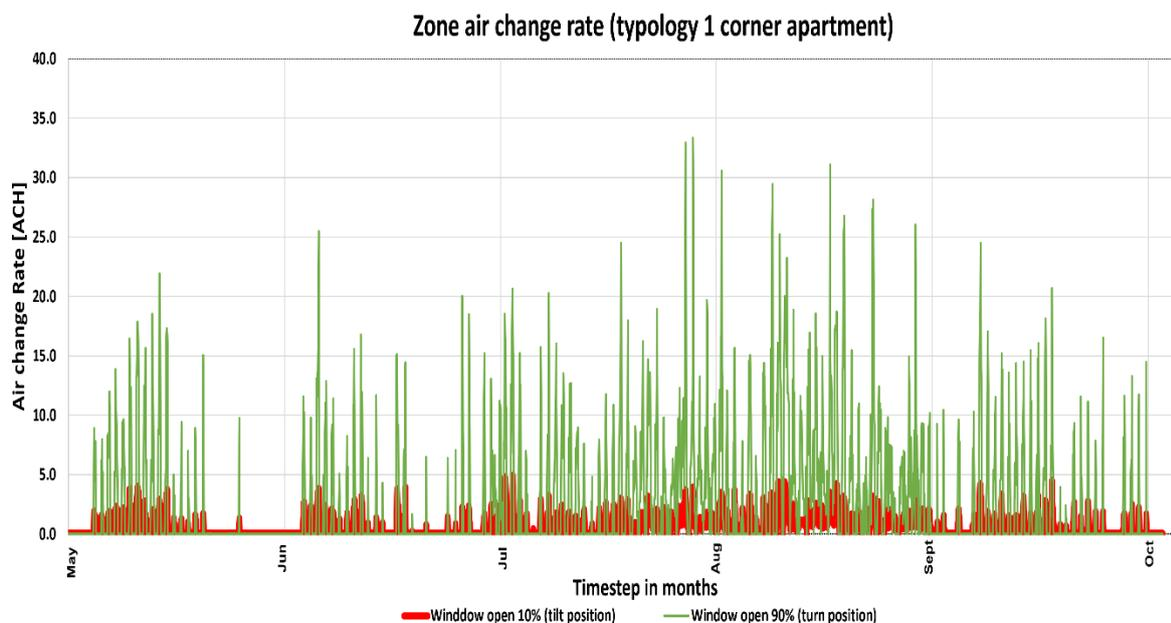
Figure 6.4. Graph showing the air change rate in the living room for the corner apartment when the windows are opened in the two positions.
