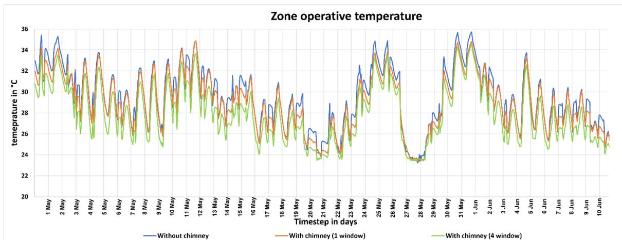
Figure 5.7. Graph showing the variation in the zone temperature when simulations were run with chimney and 10% of the window in the room was considered operable.
