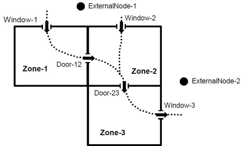
Figure 2.5. Representation of an airflow path in an airflow network diagram [17]
