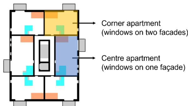
Figure 2.8. Picture showing the layout of the corner apartment and centre apartment in building typology 1.
