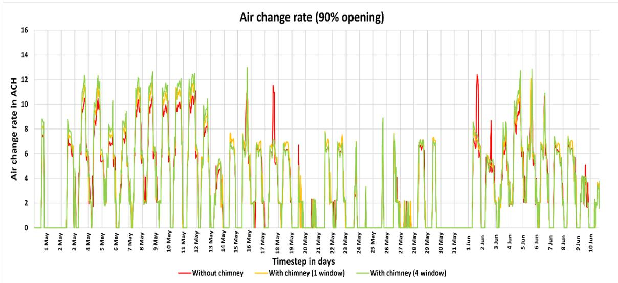
Figure 5.8. Graph showing the variation in the air change rate when simulations were run with chimney and 90% of the window in the room was considered operable.
