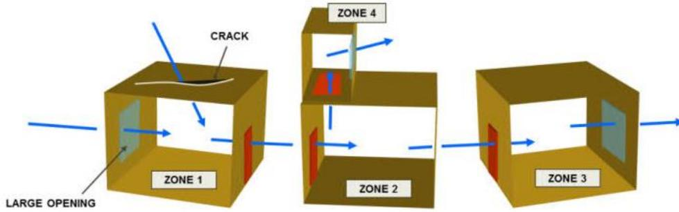
Figure 2.4. Airflow network schematic representation [6].
