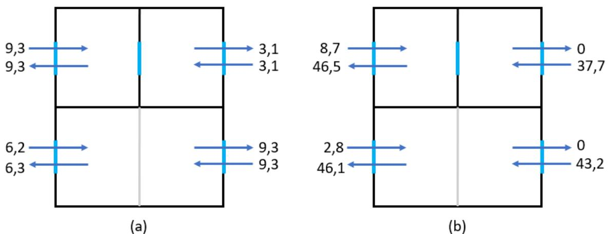
Figure 5.4. Top view diagram representation of airflow through the apertures for a multizone mode where two zones are connected by a window and two zones are connected by an airwall. (a) represents the first timestep from table 4.2 and (b) represents the last timestep from the table 4.2.
