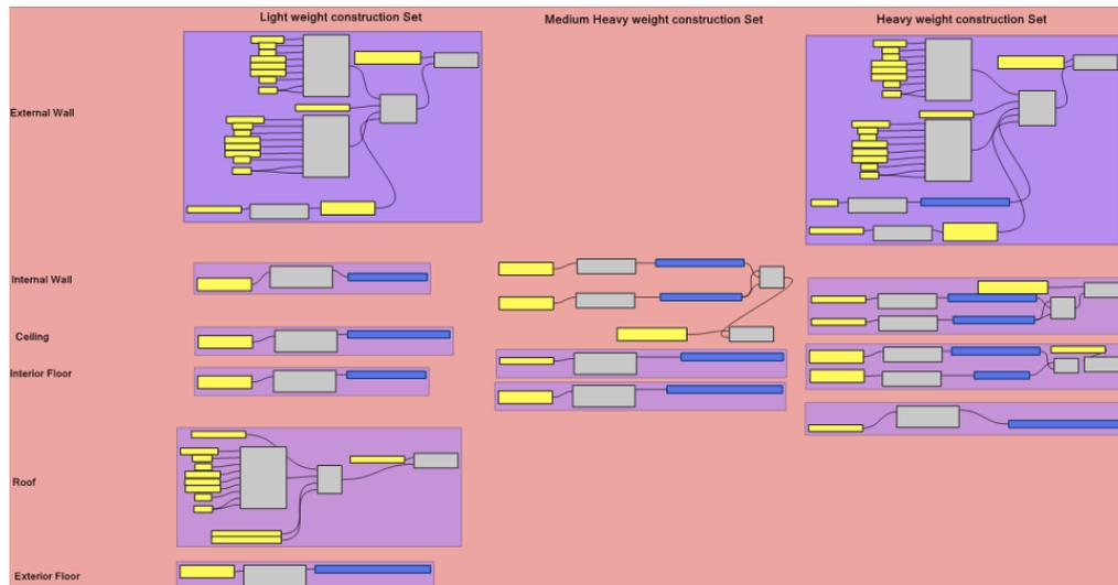
Figure 4.3. Grasshopper script showing the material definition for light, medium heavy and heavy constructions
