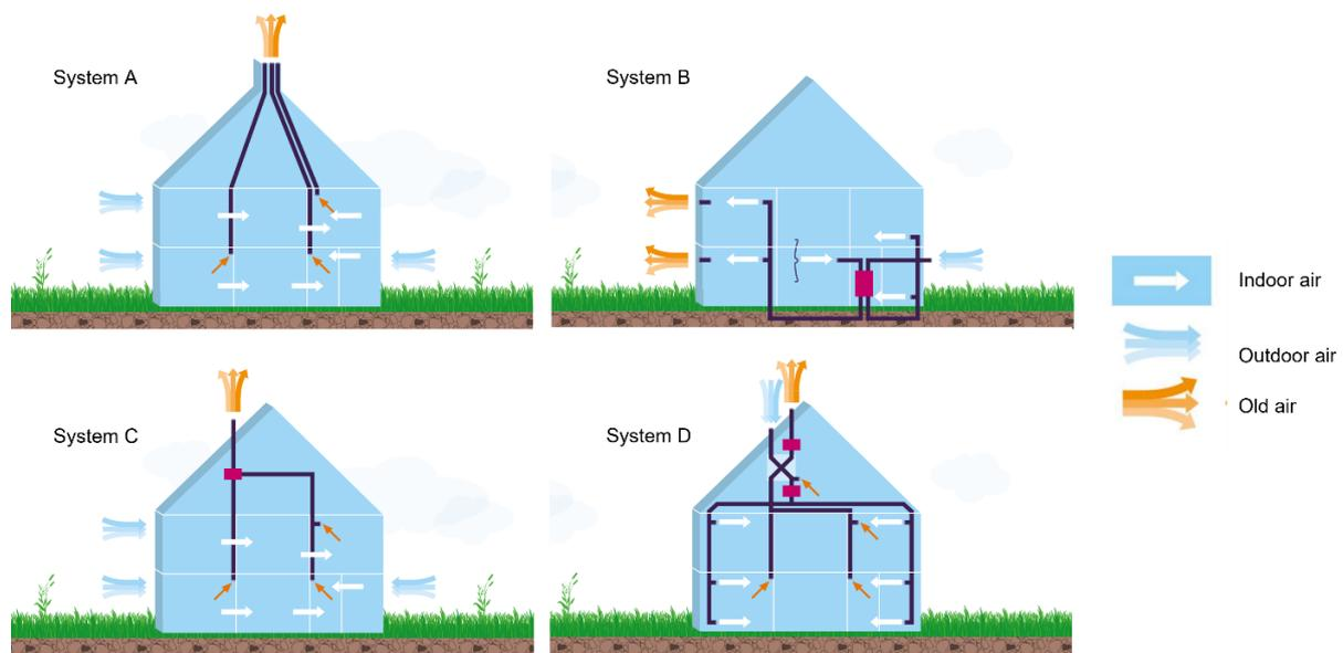
Figure 2.12. The four ventilation systems generally used in buildings [20]
