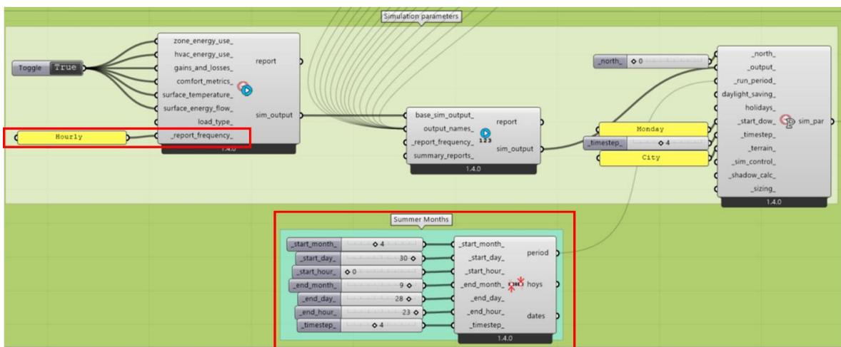
Figure 4.7. Script showing the simulation controls including the simulation period and the output report frequency
