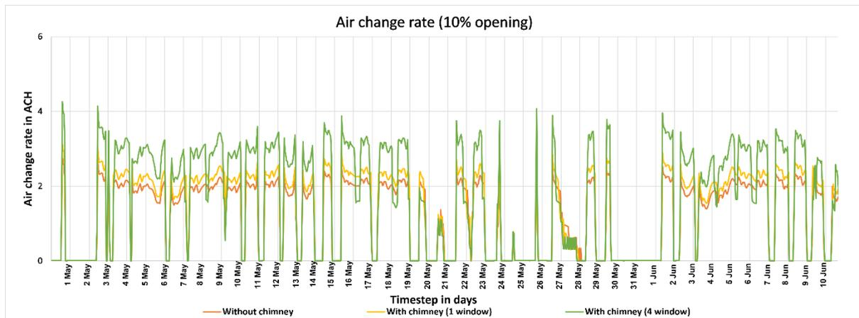
Figure 5.6. Graph showing the variation in the air change rate when simulations were run with chimney and 10% of the window in the room was considered operable.
