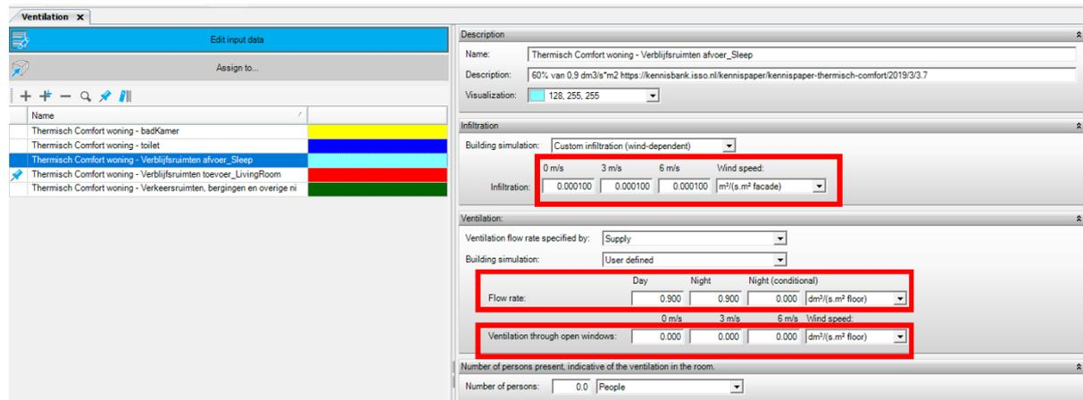
Figure 7.5. Constant mechanical ventilation rate of 0.9 l/s
