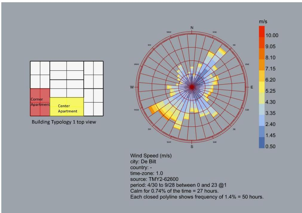
Figure 6.6. Wind rose diagram for the DE Bilt site along with the building typology 1 apartments used for simulation shown.
