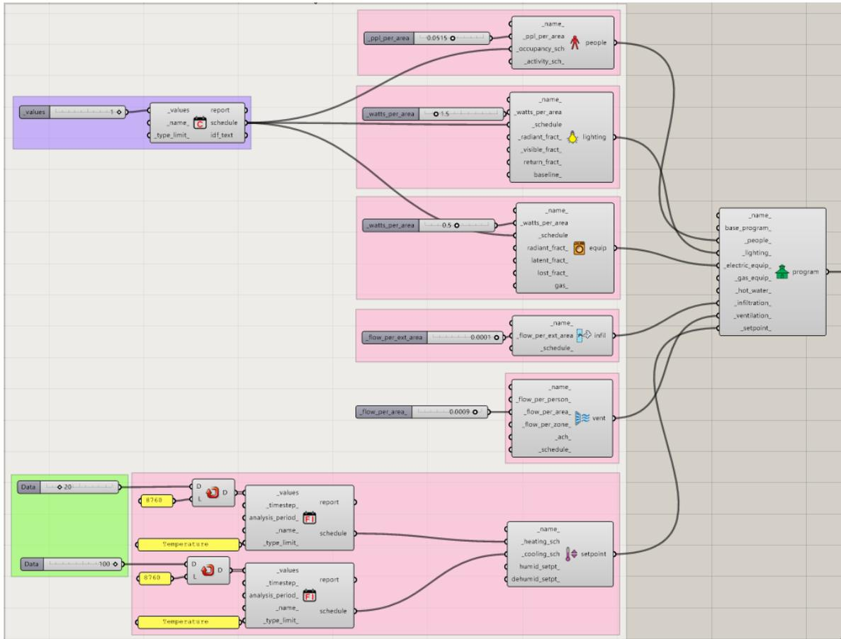
Figure 4.4. Program type definition for internal heat loads, mechanical ventilation rate and heating and cooling setpoints.
