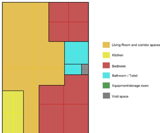
Figure 2.11. Building Typology 2 gallery apartment illustration showing the different zones
