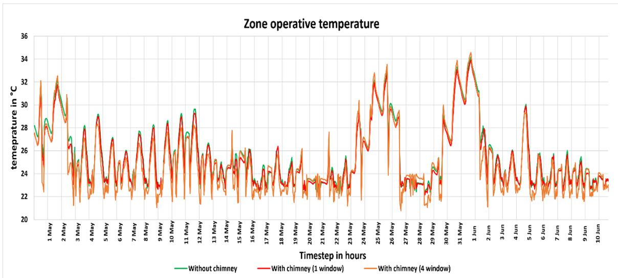
Figure 5.9. Graph showing the variation in the zone temperature when simulations were run with chimney and 90% of the window in the room was considered operable.
