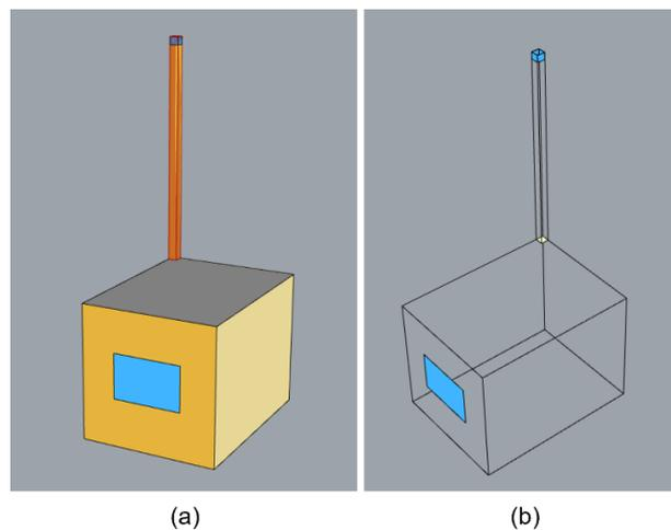
Figure 5.5. (a) Chimney with four windows connected to a zone with a single window on the facade. (b) shows the airwall connection with the roof and the apertures on the zone and the chimney.
