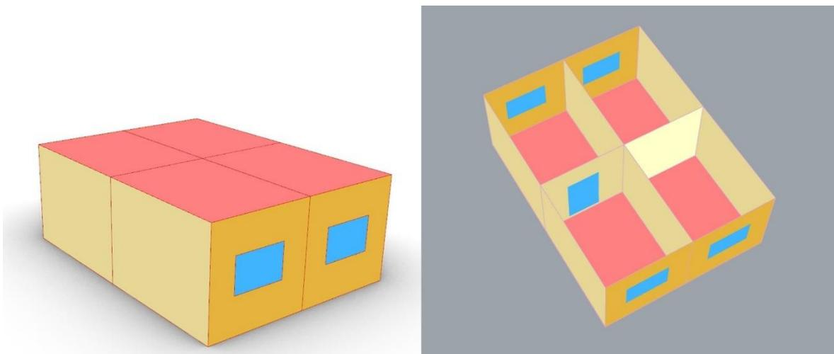
Figure 5.3. Multizone model with four zones for testing. Each zone having an exterior window. Two zones are connected by an internal aperture and the other two zones are connected by airwall.
