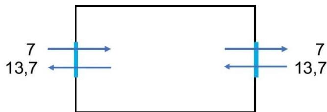
Figure 5.2. Diagram representation showing the plan of the single zone model with airflow through the apertures
