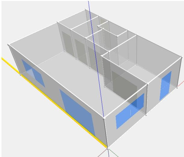
Figure 7.1. VABI geometry for corner apartment
