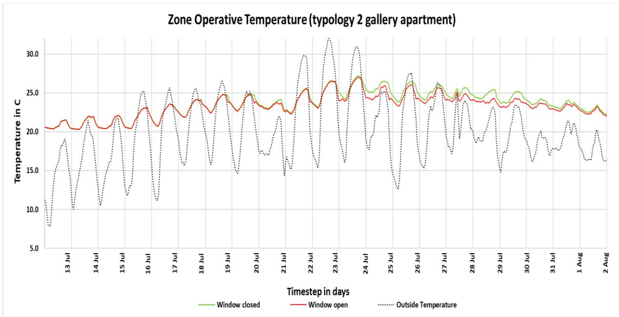
Figure 6.3. Zone operative temperature of gallery apartment for three cases. The blue line represents the zone temperature when the windows are closed for the whole time. The orange line represents the zone temperature when the windows are opened. (full graph in Appendix D)
