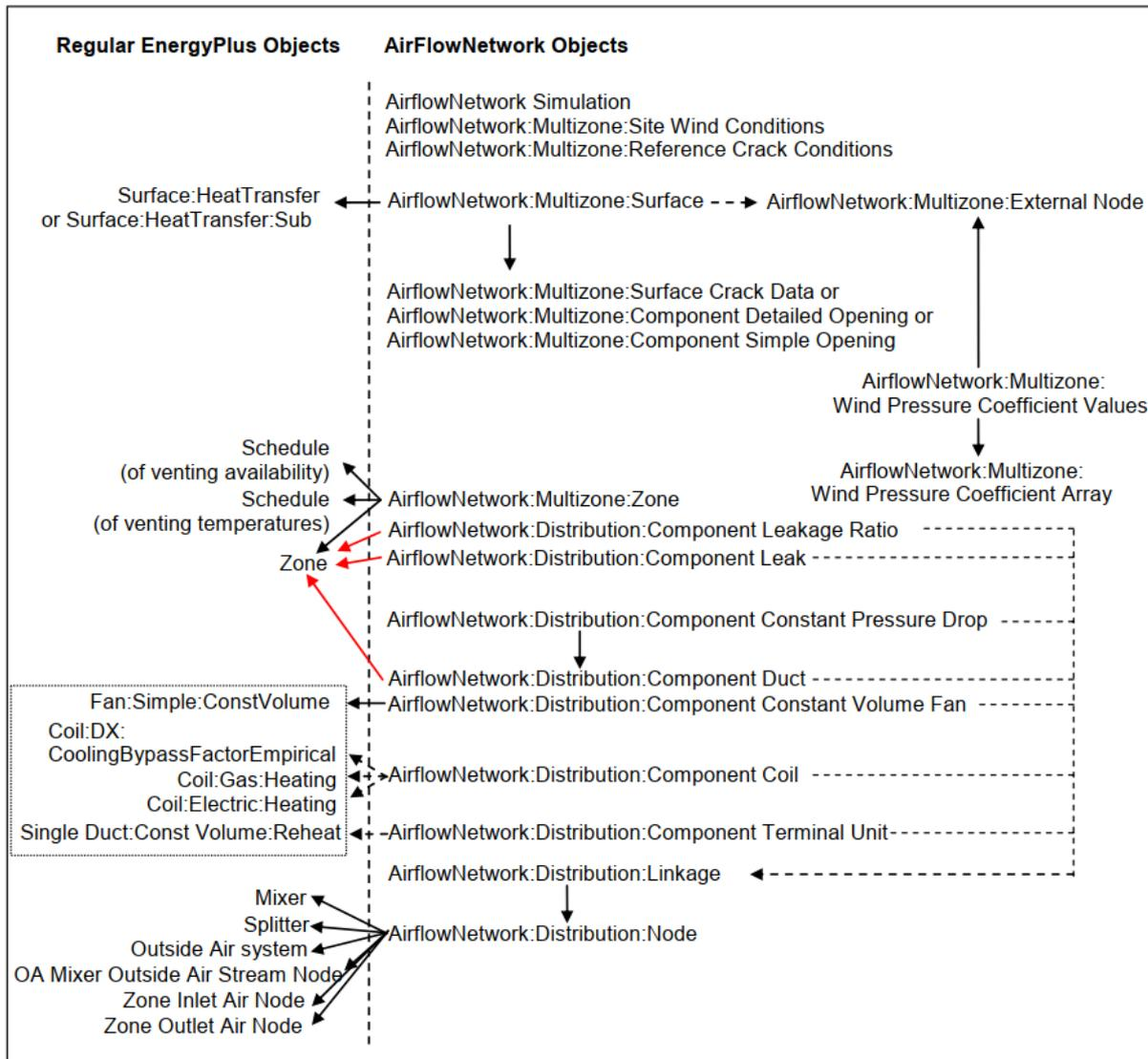
Figure 2.6. Energyplus objects and the associated airflow network objects. Arrows from object A to object B shows that object A references object B [17]
