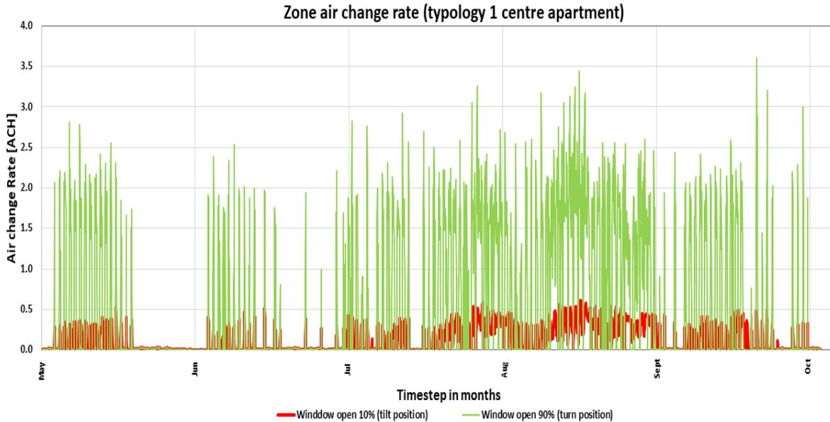
Figure 6.5. Graph showing the air change rate in the living room for center apartment when the windows are opened in the two positions.
