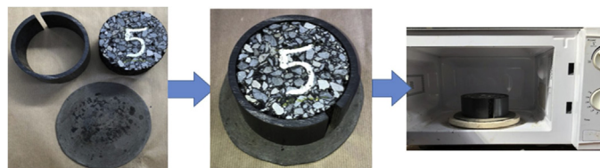
Fig. 3. Microwave healing test system set up.
