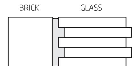
Furthermore, the orientation of stacked glass elements was identified as a critical factor influencing the shear strength and ductility of joints involving brittle materials. To optimize performance, a combination of interlocking geometric forms and surface roughness was proposed. Specifically, employing an interlocking shape with a more layered configuration was recommended.
