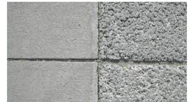
Figure 54: Non-porous concrete [left] versus porous concrete [right]. Source: (Florida association of country engineers & road superintendents)
