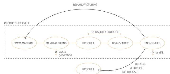
Figure 6: Illustration of recycling opportunities with design for disassembly.
