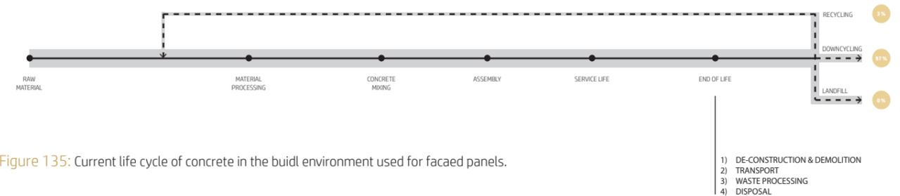
Figure 135: Current life cycle of concrete in the build environment used for facade panels.
