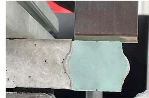
Figure 129: Interlocking shape contributes to movement constraints.
