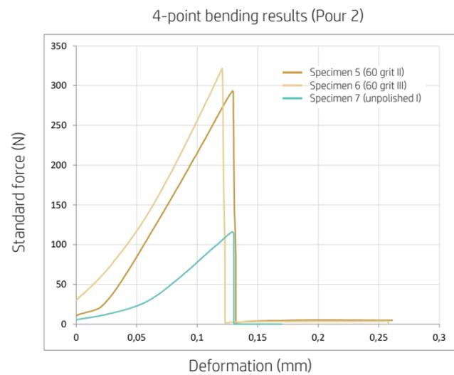
Figure 99: Force-Deformation diagram of the 3 specimens (Pour #2)
