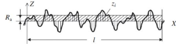
Figure 82: Surface profile and  $R_a$ . Source: (Hong et al., 2014)
