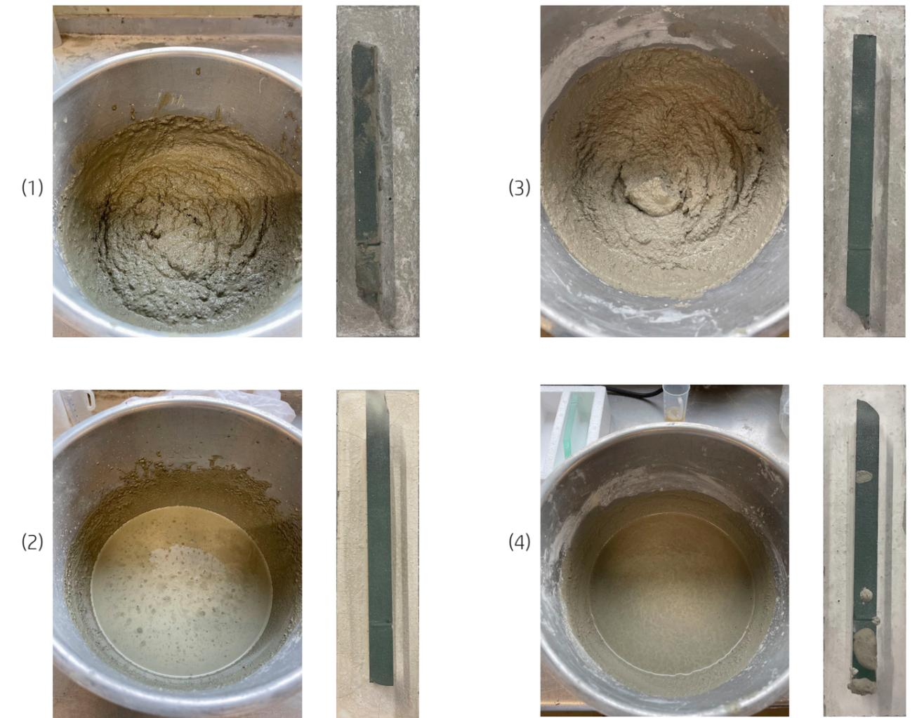
Figure 60: The four different concrete workability after mixing the the composition. In formulations incorporating Glenium as a plasticizer, the resulting mixtures exhibit significantly higher fluidity.
