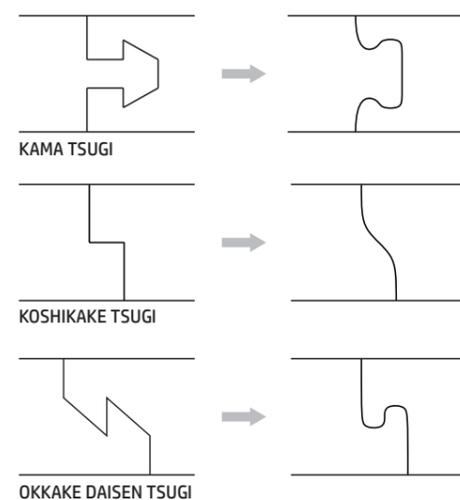
Figure 69: interlocking forms retrieved from old Japanese timber connections.
