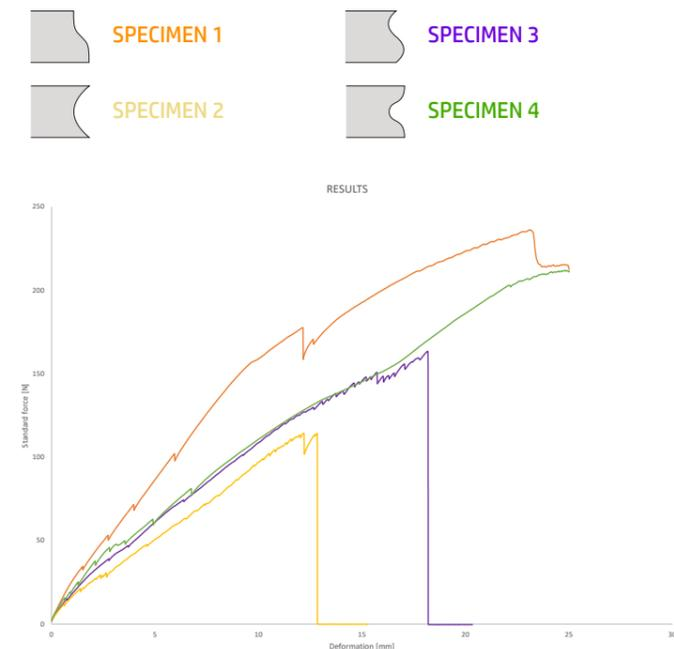
Figure 79: Test results of 3-point bending test of the interlocking specimens.
