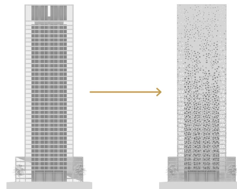
Figure 116: Design consideration of a more open facade at a lower height and. Reducing the interfaces in the top area of the building. Downside is a view obstruction.
