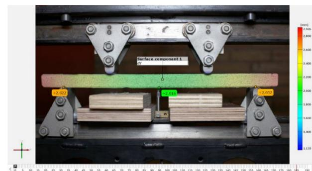
Figure 127: Bristogianni (2022) showed how to measure the displacement in the Y direction, by analyzing the images using the *GOM Correlate* software.
