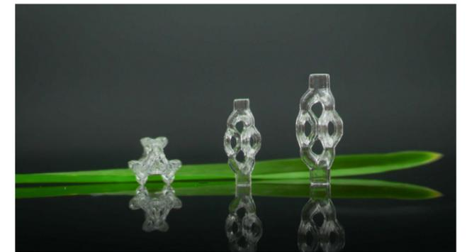
Figure 46: Glass microstructures developed by 3D printing technology. Source: (Berkeley engineering)
