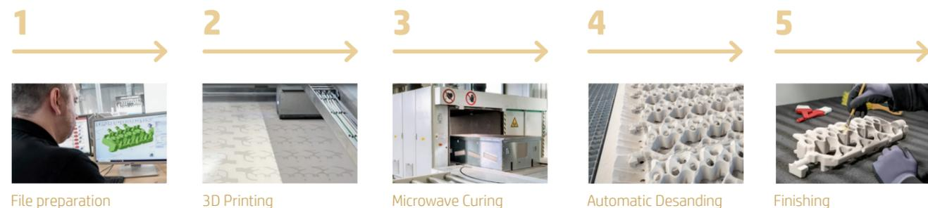
Figure 140: Production Line of a 3D printed sand mould by (ExOne, 2021).
