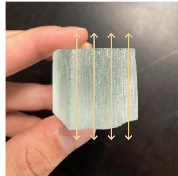
Figure 123: Horizontal polishing lines are visible due to one-way polishing.
