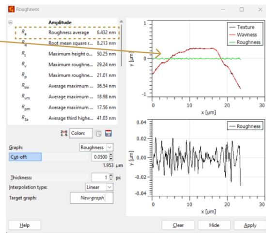
Figure 105: Measurement of the average surface roughness of a  $25 \times 25 \mu\text{m}$  area.
