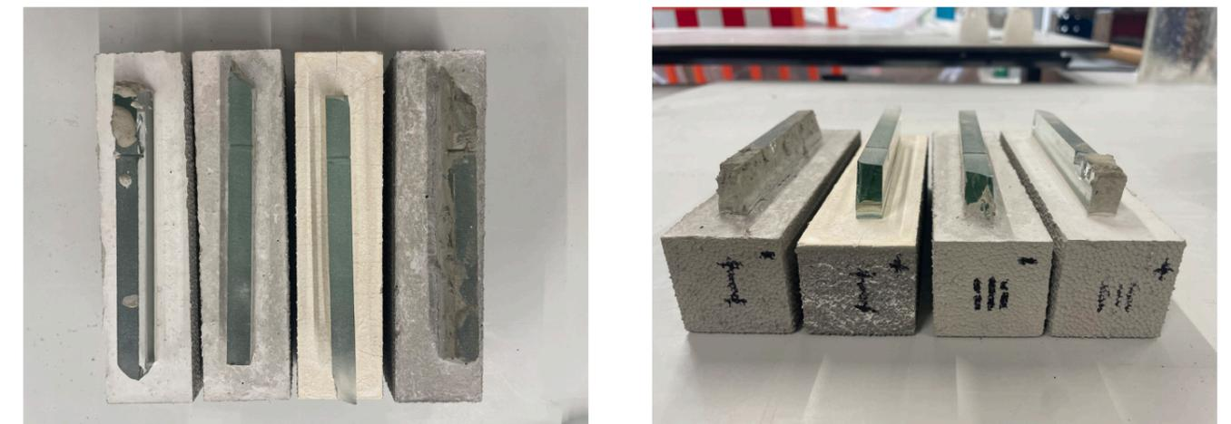
Figure 61: 4 different concrete compositions after 7 days of curing. It can be observed that with the addition of I+ (composition 2), the overall concrete has significantly shrunk due the plasticizer.
