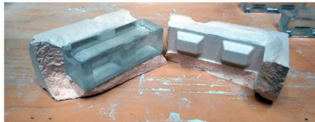
Figure 43: Disposable silica-plaster mould. Source: (Oikonomopoulou, 2019)
