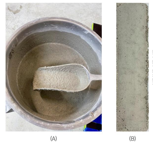
Figure 94: Concrete mixture of pour #1. The workability was too fluid. The disintegrated upper layer, consisting of numerous air bubbles and water from the cured concrete (B), is evident in the mix (A).
