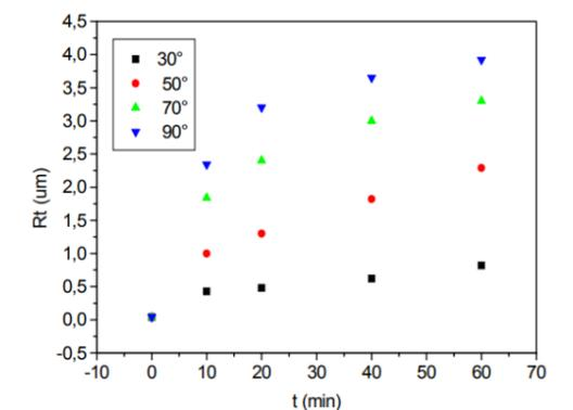
Figure 87: Bousbaa (1998) observed an increased surface roughness over time
