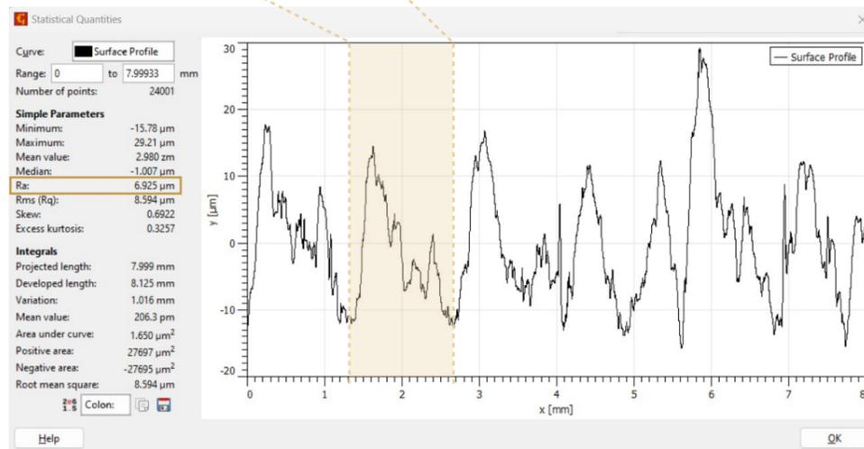
Figure 111: Top: surface roughness calculation of one peak over a distance of 1,35 mm ( $R_a = 6,356 \mu\text{m}$ ). Bottom: Average surface profile over a length of 8 mm with an average surface roughness of ( $R_a = 6,935 \mu\text{m}$ ).
