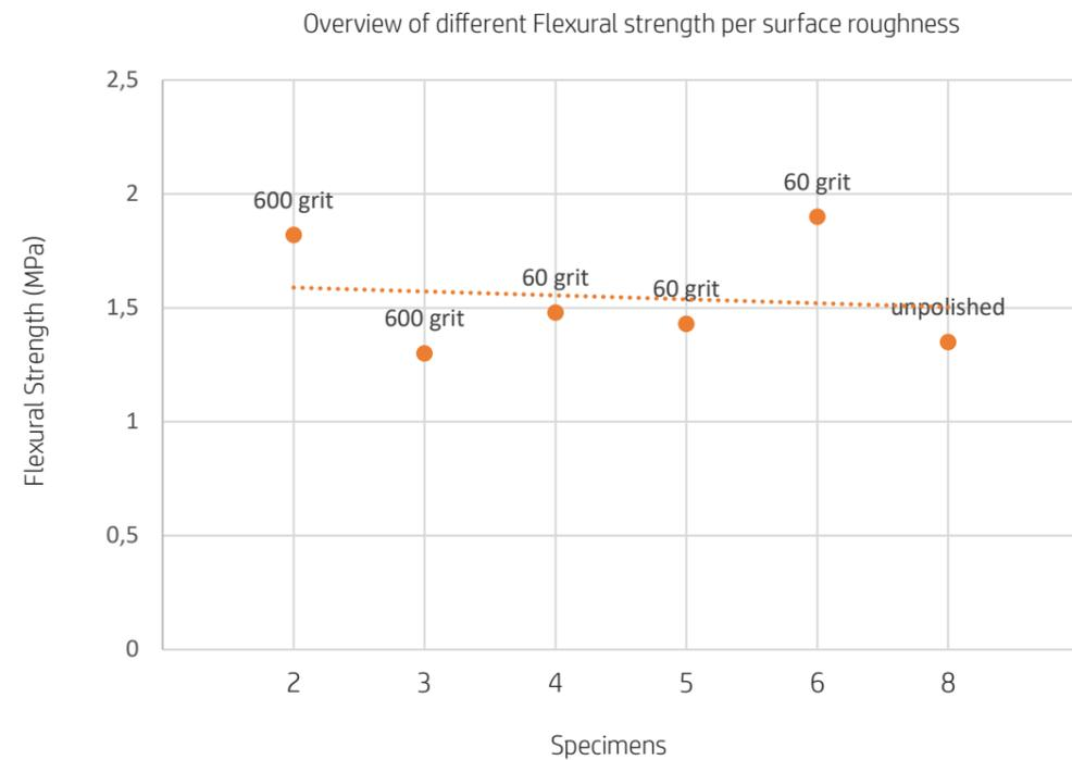
Figure 103: Overview of different Flexural strength per surface roughness
