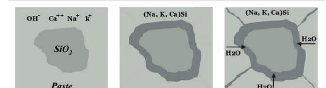
Figure 16: Sequence of Alkali-Silica Reaction (ASR) in concrete. Source: (Al-Neshawy, 2013)
