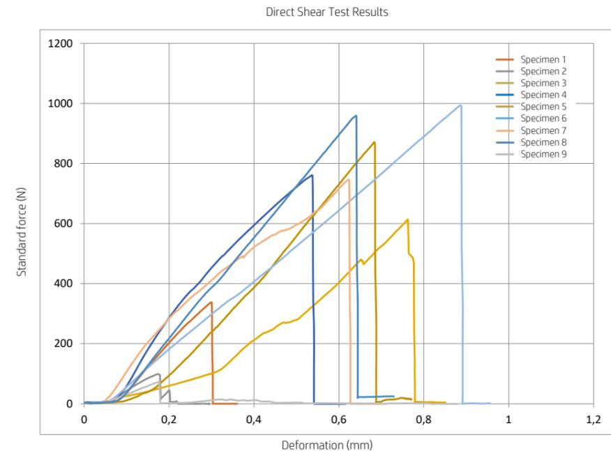
Figure 130: Table of test results of the nine specimens after direct shear test.
