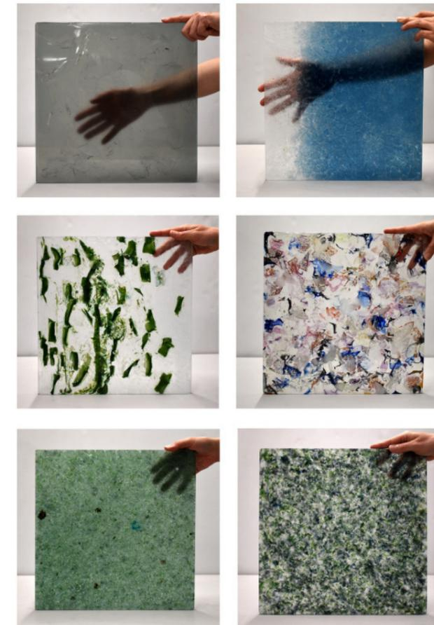
Figure 135: Bristogianni (2022) showing the possibility of using recycled glass waste cullets for kiln-casting glass panels.
