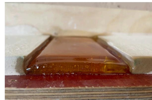
Figure 75: Left: Instead of the plaster sticking to the edge of the sugar glass, it is gradually absorbed. Right: Because sugar glass adheres too firmly to the mold, detaching is not possible, resulting in the sugar glass breaking.
