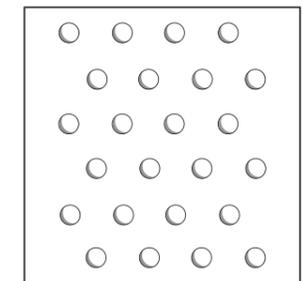
Figure 135: A dimpled surface increases the contact area and still keeps a round shape which is preferred for brittle materials and in cast glass manufacturing.
