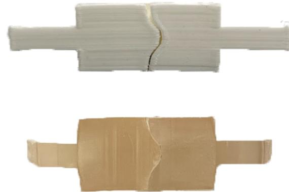
Figure 75: Top: layered FDM printed interlocking form. Bottom: Higher accuracy SLA printed interlocking form.
