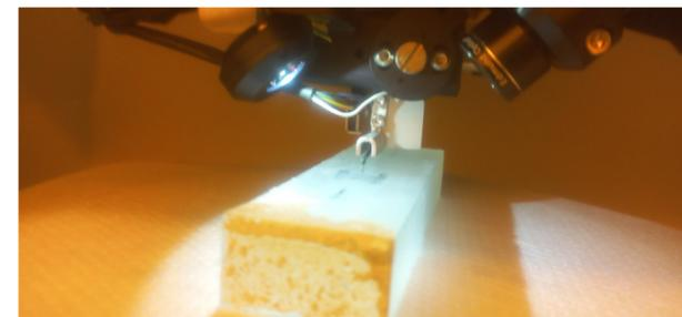
Figure 108: Probing an unpolished cast glass sample with a Dektak profilometer.
