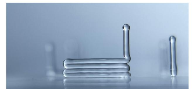
Figure 48: Single multi-layer wall with free-standing print. Source: (Nobula3D)
