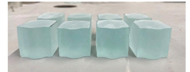
Figure 119: Casted interlocking belly shaped glass elements.
