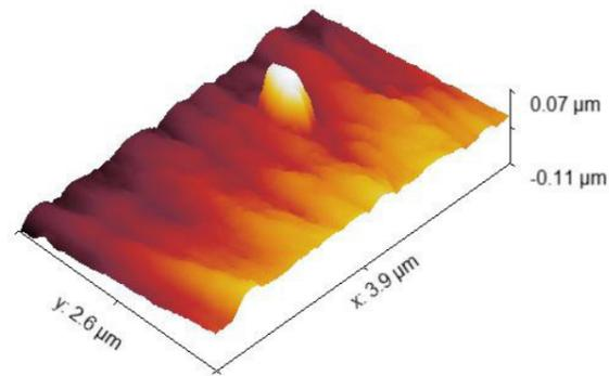
Figure 106: Roughness profile measured on  $3.5 \times 3.5 \mu\text{m}$  surface with a surface imperfection. Likely a gypsum particle that remained stuck to the glass surface from the Crystalcast mould.
