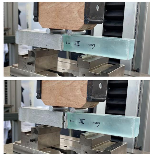
Figure 100: All specimens broke in the interface with a clear breakline just like Specimen 3 shown above.
