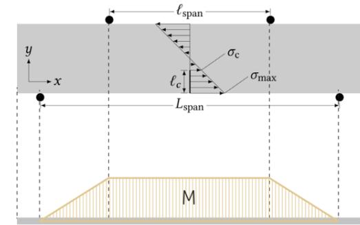
Figure 97: Visualisation of the parameters for the formula of maximum bending stress in a 4-point bending set-up and the corresponding bending moment diagram (Doitrand et al., 2021).
