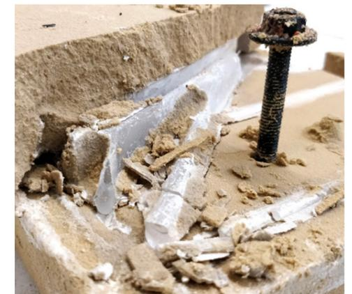
Figure 140: Avoid using bolts and screws. They will fuse and can't be removed, making the demoulding process impossible (Bhatia, 2019).
