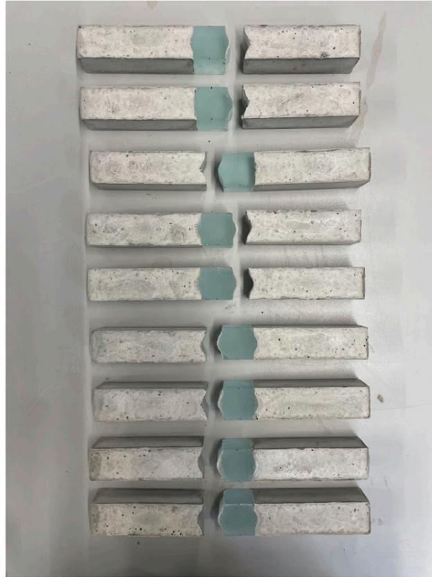
Figure 122: Detachment of the concrete parts after demoulding the specimens.
