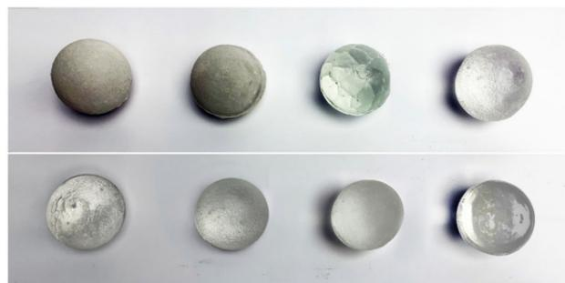
Figure 45: Different coatings for glass casting on 3DPSM. Source: (Ioannidis, 2023)
