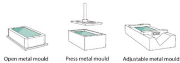
Figure 42: Three types of permanent moulds. Source: (Oikonomopoulou, 2019)
