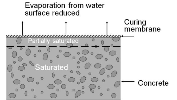
Figure 53: Water curing of concrete scheme. Source: (www.aboutcivil.org)
