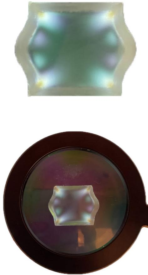
Figure 120: Polarised pictures of the belly shape cast glass element, introducing the highest internal stress in the 90 degree angles and not in the belly.
