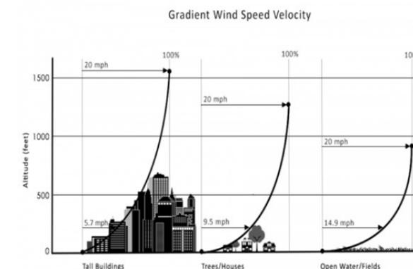
Figure 116: Wind velocity increase in height.
