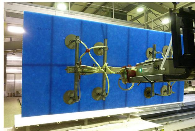
Figure 135: Maximum panel size (3500 x 1500mm) made from 100% recycled glass cullets by MAGNA Glaskeramiek.
