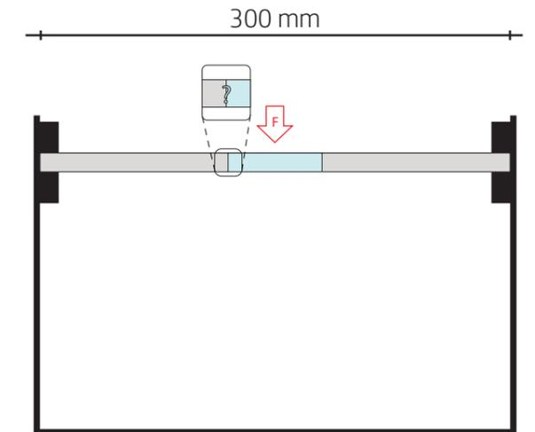
Figure 73: Test set up for testing different interlocking forms.
