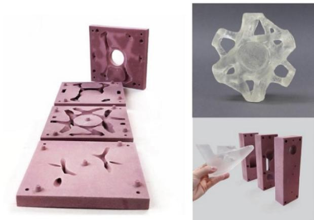
Figure 44: 3D printed sand moulds. Source: (Damen; Bhatia, 2019)
