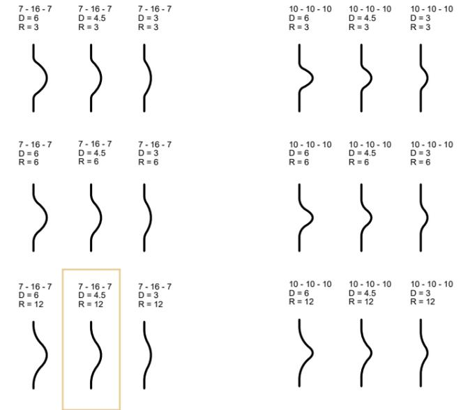
Figure 118: only a small part of various belly shape forms with different height, width and rounding radius.
