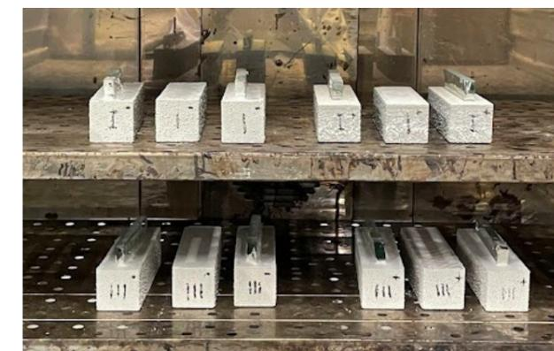
Figure 64: Specimens are placed in oven at 80 °C degree for 4 hours.
