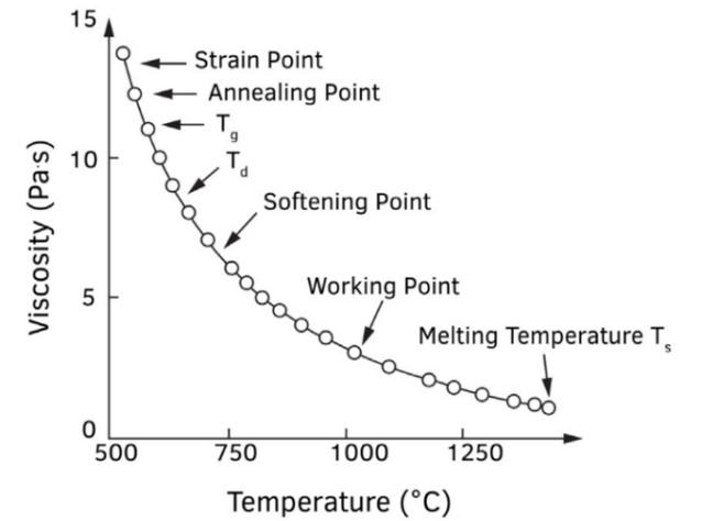
Figure 40: Viscosity curve as a function of temperature for soda-lime glass. Source: (Shelby, 2005)
