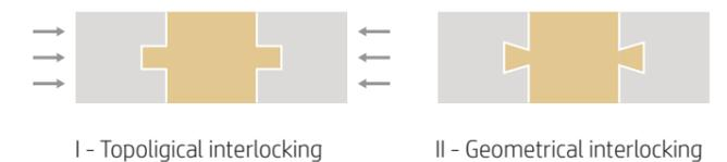
Figure 66: Visualisation of topological and geometrical interlocking
