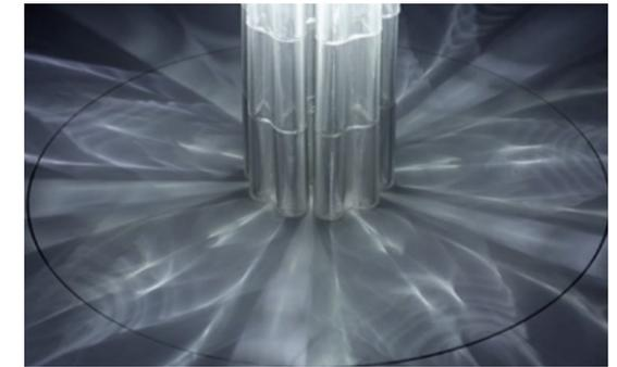
Figure 29: Large-size glass column printed by G3DP2 (invented by MIT). Source: (Inamura, 2018)
