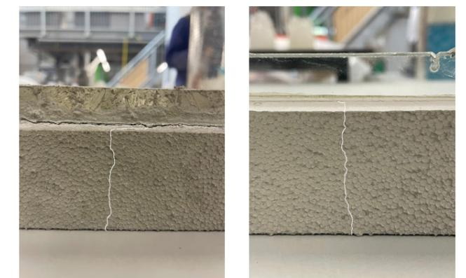
Figure 65: Cracks found in the bulk of the concrete bij concrete composition #1 (left) and #3 (right).
