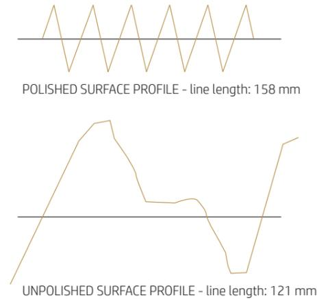
Figure 110: Different surface profiles of polished and unpolished cast glass elements with correspondnig line lengths.
