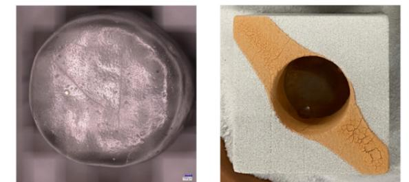
Figure 140: Arkopal B 5 as most promising coating on quartz sand mould, with an annealing schedule at 807 °C conducted in thesis work of (Ioannidis, 2023).
