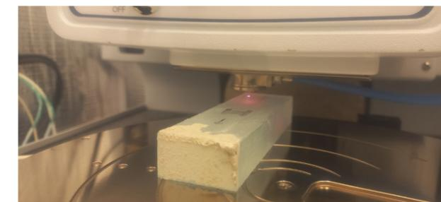
Figure 104: Probing an unpolished cast glass sample with an AFM
