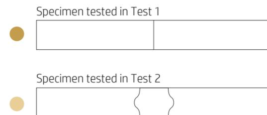
Figure 130: Overview of the two 4 Point bending tests. Test 1 resulted in a higher average flexural strength but only consists one interface. Test 2 results in a lower interface bending strength.
