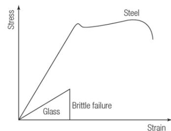
Figure 23: Stress-strain curve showing brittleness of glass compared to steel. Source: (Weller, 2009)
