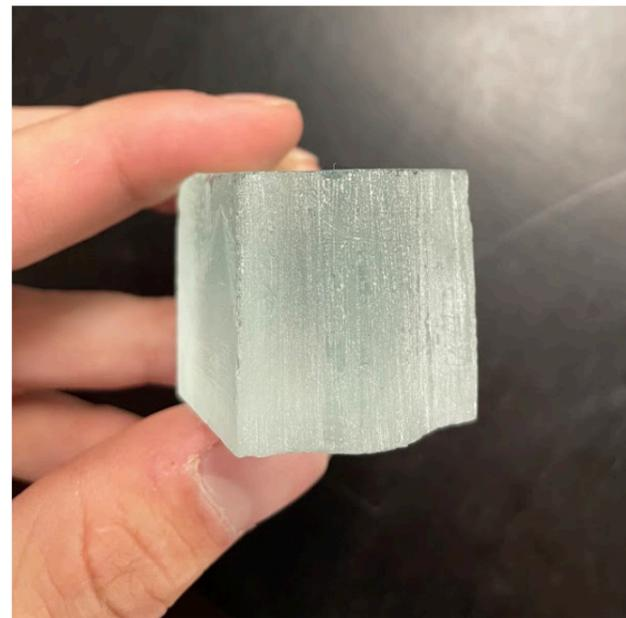
Figure 121: Polished interface surface with grit 60.
