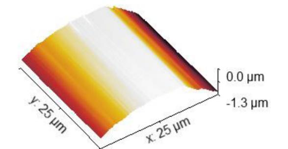
Figure 103: Top: surface profile of an unpolished cast glass element measured on a 25x25 micrometers area. Bottom: 3D visualisation of the surface profile.
