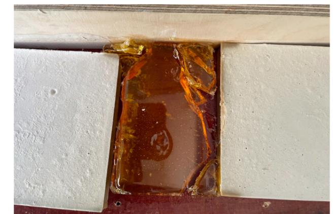
For the search for the best interlocking form, a different design setup has been devised where the various shapes are inserted as a setup piece into a wooden panel to subject them to different forces.
