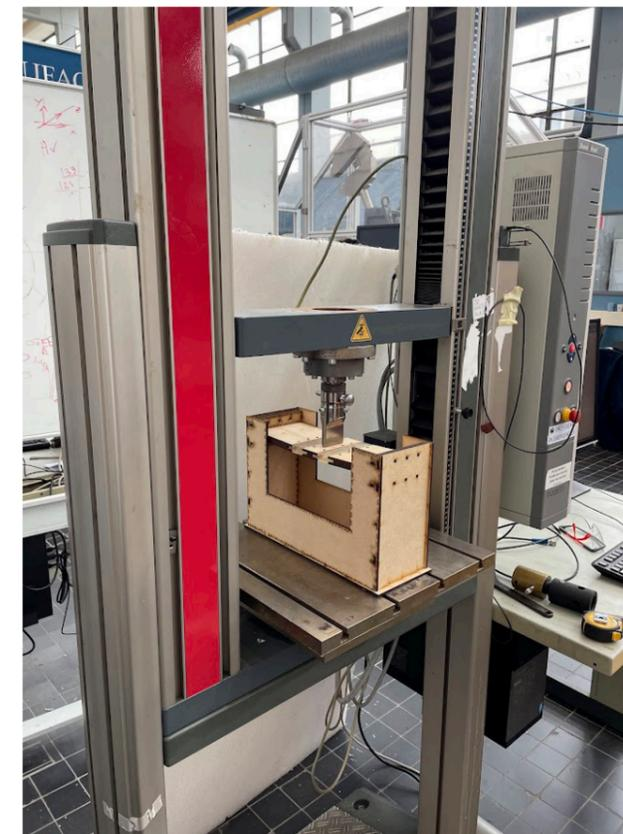
Figure78: point load test with a clamped specimen is conducted at ME with Fred Veer.
