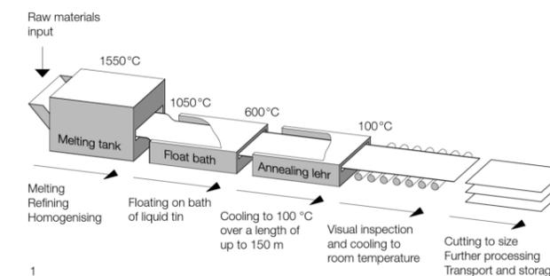
Figure 28: Schematic illustration of the float glass process. Source: (Weller, 2009)
