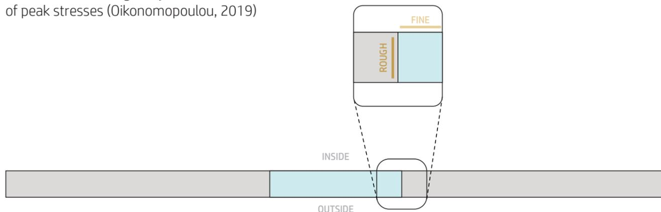
Figure 88: A cross-section of a hybrid panel consisting of concrete and glass, where the interface between the materials requires a rough surface, while the exterior demands smoothness.
