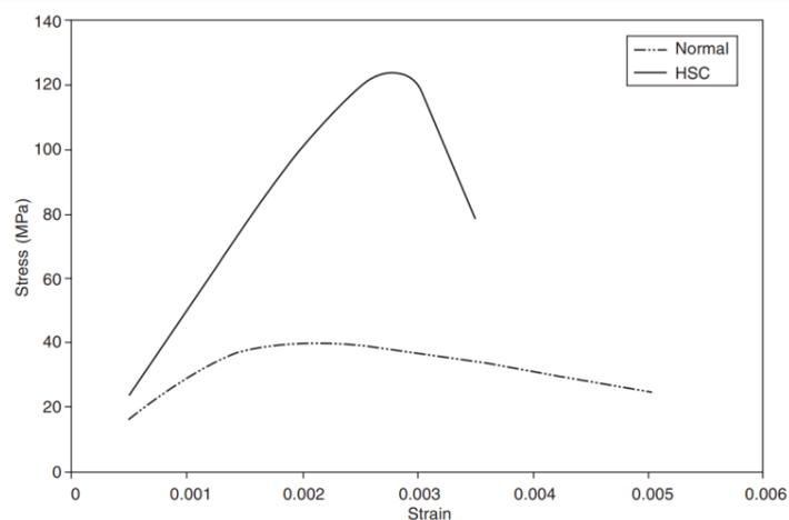
Figure 55: Comparisson of a stress-strain curve between NSC and HSC. Source: (ADD)
