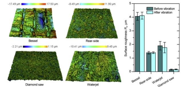
Figure 85: surface topographies and average roughness of different glass cutting technologies (Dudutis, 2020)
