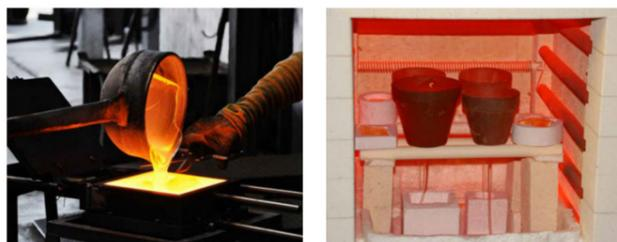
Figure 32: Primary casting [left] and secondary casting [right]. Source: (Oikonomopoulou, 2019)
