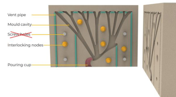
Figure 140: Design considerations of a 3D printed sand mould implemented for a final design (Bhatia, 2019).
