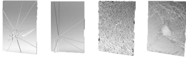
Figure 37: Strength type of glass. From left to right; Annealed, Heat-strengthened, Fully tempered and Laminated. Source: (Weller, 2009)
