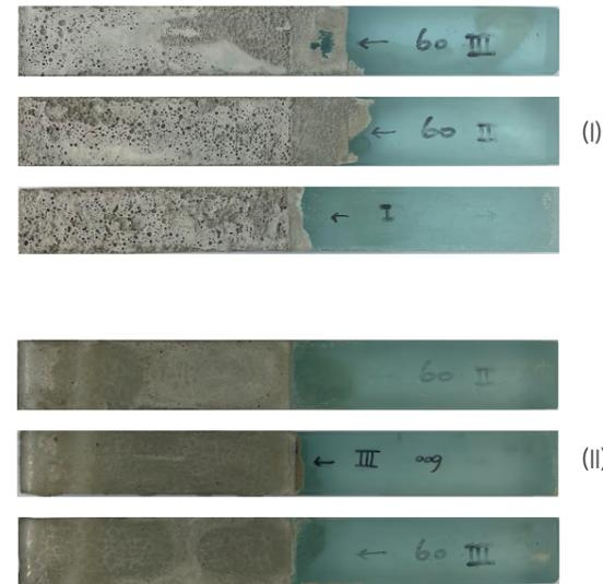
Figure 95: In the second pour, it is evident how the concrete has disintegrated, creating a brittle top layer of concrete (I) compared to well-mixed homogeneous concrete (II).
