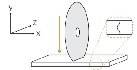
Figure 86: Illustration of the drawback of cutting cutting technologies (diamond saw) when using 3D cross-sectional forms.
