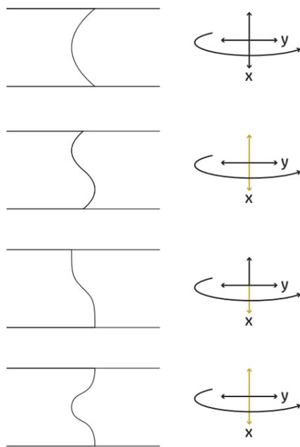
Figure 71: interlocking forms retrieved from old Japanese timber connections.
