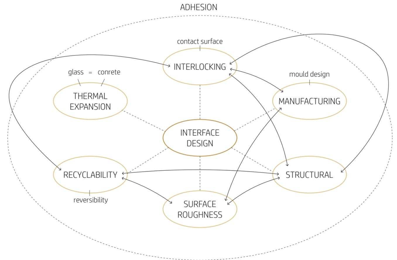
Figure 18: Illustration of different design aspects for creating a hybrid interface.
