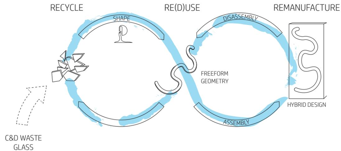
Figure 135: Closed loop diagram for the glass part of a hybrid facade panel.
