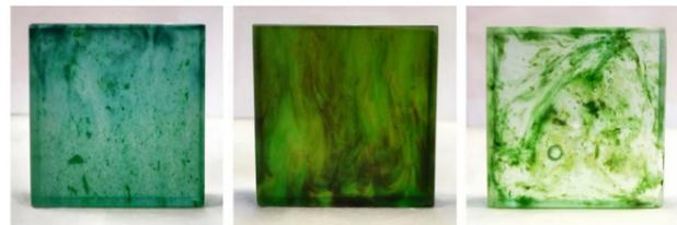
Figure 25: Glass prototypes made from recycled car windshields (left), containers (middle) and oven-doors (right). Source: (Bristogianni, 2022)
