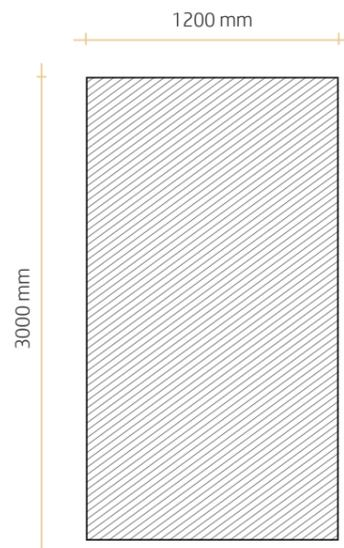
Figure 114: Dimensions of a facade panel with a floor to floor height.
