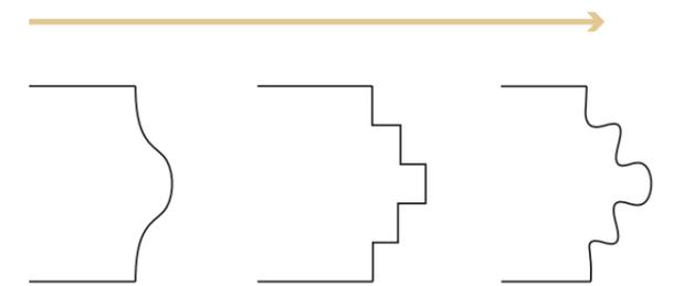
Figure 135: Example for a new interlock design based on the findings of the experimental part.
