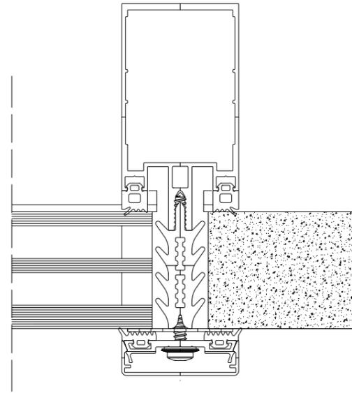
Figure 136: Detail of a curtain wall system with regular triple glazing on the left and a hybrid facade panel on the right.
