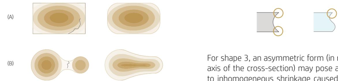
Figure 70: Shape limitations for cast glass elements. Edited from (Damen, 2019). (A): Sharp edges will increase residual stress, thus premature failure. (B): A connector/key with a considerably smaller cross-sectional area also leads to increased stress and high risk of premature failure.
