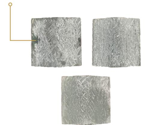
Figure 127: Increasing the roughness manually with a dremel on the glass surface of an interlocking glass element.
