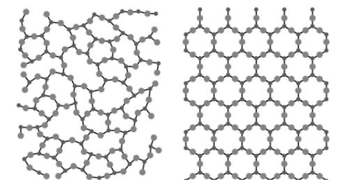
Figure 21: Molecular structure amorphous solid; glass [left] and crystalline solid; quartz [right]. Source: (Weller, 2009)
