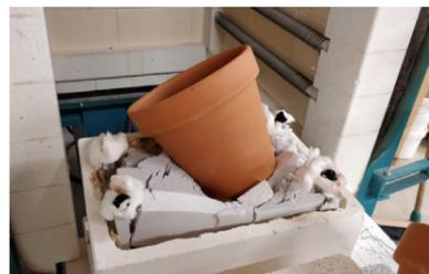
Figure 140: Breakage of the sand mould during firing due the weight of the flowerpot and the weaker sand mould (Bhatia, 2019).
