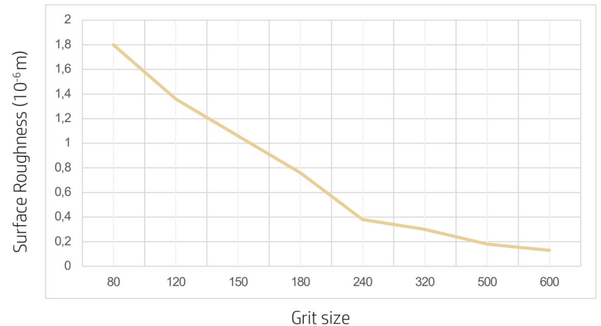
Figure 89: A table displaying the correlation between surface roughness corresponding to various grit sizes used for polishing cast glass.
