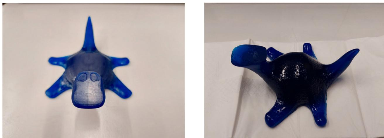
Figure 90: A layered FDM printed wax model (left) and a smooth SLA printed wax-based photosensitive resin model (right). Photo by: Anna Maria Koriari (2022)
