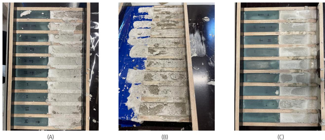
Figure 93: Different types of pouring against the glass, where the concrete composition remains the same but various mixing and compaction procedures are employed. (A): Test pour 1, (B): Test pour 2, and (C): Test pour 3.
