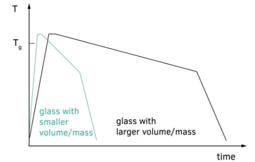
Figure 41: Annealing time for different volumes of glasses. Source: (Oikonomopoulou, 2019)
