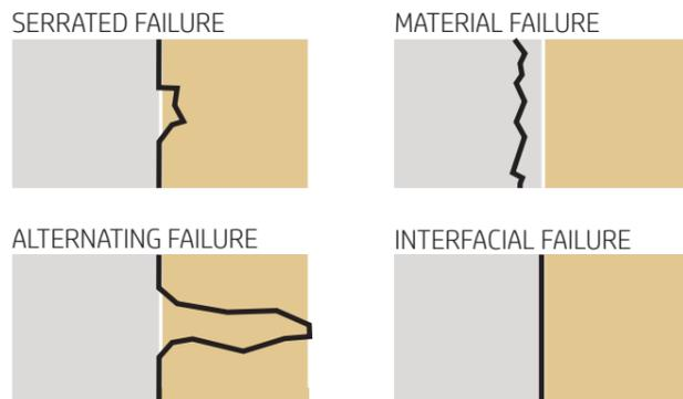
Figure 126: Schematic illustration of different failure modes possible after direct shear test.
