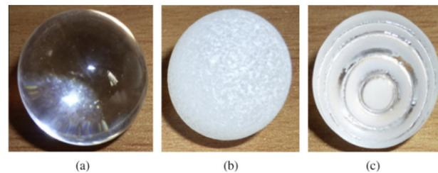
Figure 83: Different surface roughness of HBG aggregates; (a) polished surface with  $R_o = 24.0 \mu\text{m}$  | (b) sandblasted surface with  $R_o = 48.3 \mu\text{m}$  | (c) notched surface with  $R_o = 259.6 \mu\text{m}$  | Source: (Hong et al., 2014)
