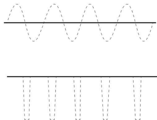
Figure 112: Top: A consistent ribbed surface profile. Bottom: By making incisions, also a consistent surface profile is created. Both can be beneficial in terms of adhesion.
