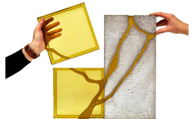
Figure 10: Feasibility study by ReStruct group TU Delft of a concrete-glass panel.
