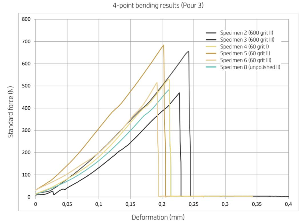
Figure 101: Force-Deformation diagram of the 6 specimens (Pour #3)
