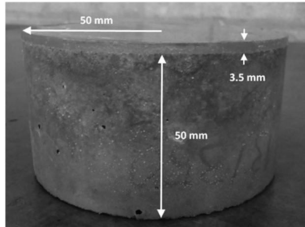
Figure 13: Prototype for testing interfacial bond strength. Source: (Gilabert et al., 2016)
