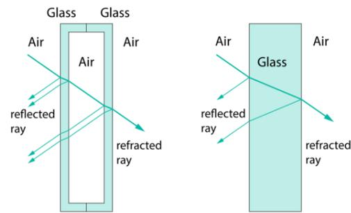
Figure 22: Transition of light through a hollow glass block and solid blocks. Source: (Oikonomopoulou, 2019)
