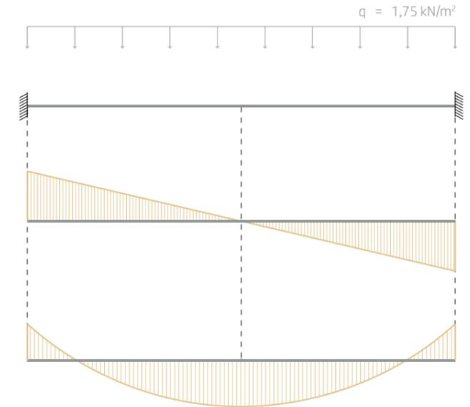
The support system with both fixed ends shows the most favourable condisation. The panel allows 'moment free' places in the panel. The maximum bending is at the ends of the panel. Considering that it is preferable to have the interface in the middle of a panel rather than entirely on the outer edge, this is a favorable situation. In general, this support system experiences the least bending.
