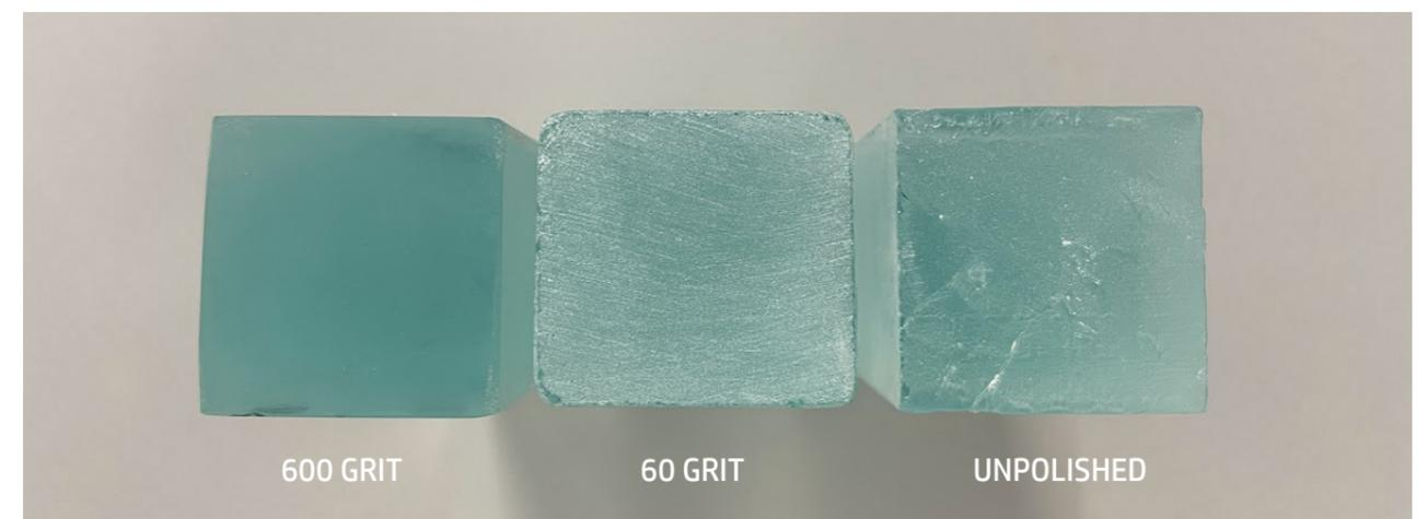
Figure 92: Three different glass surface roughnesses.
