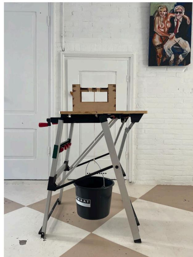
Figure 77: Left: test set-up for testing the interlocking strength with a bucket filling up with water. The interlocking strength was higher than the water capacity of the bucket.
