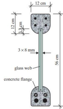
Figure 84: Pre-treated glass web in glass-concrete composite for improved structural performance. Source (Freytag, 2014).
