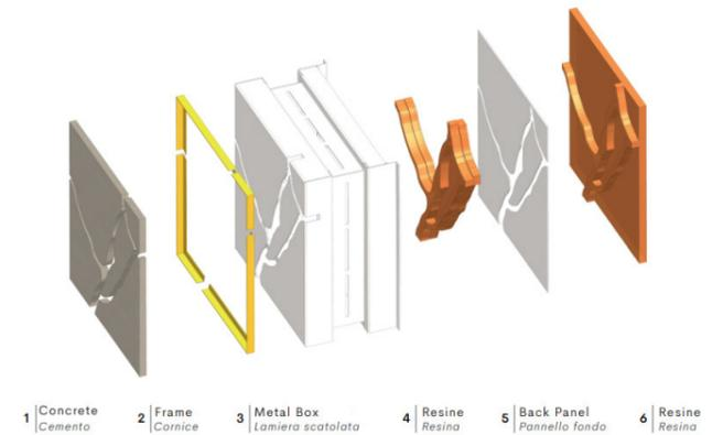
Figure 9: Feasibility study by ReStruct group TU Delft of a concrete-glass panel.
