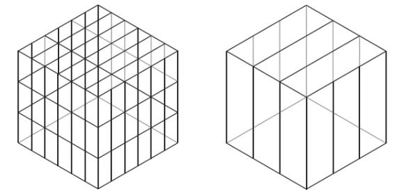
Figure 34: By using larger panels, Apple's store using just 15 panes instead 90. Source: (Apple)
