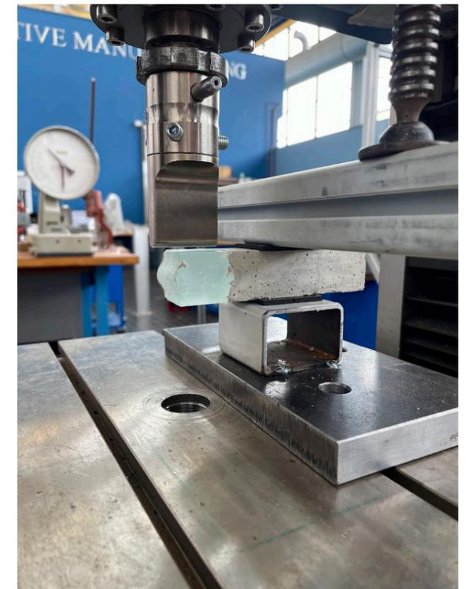
Figure 127: Left: 4 point bending test with an interlocking glass pieces surrounded by concrete. Right: A direct shear test by clamping the concrete part and applying pressure on the glass part.
