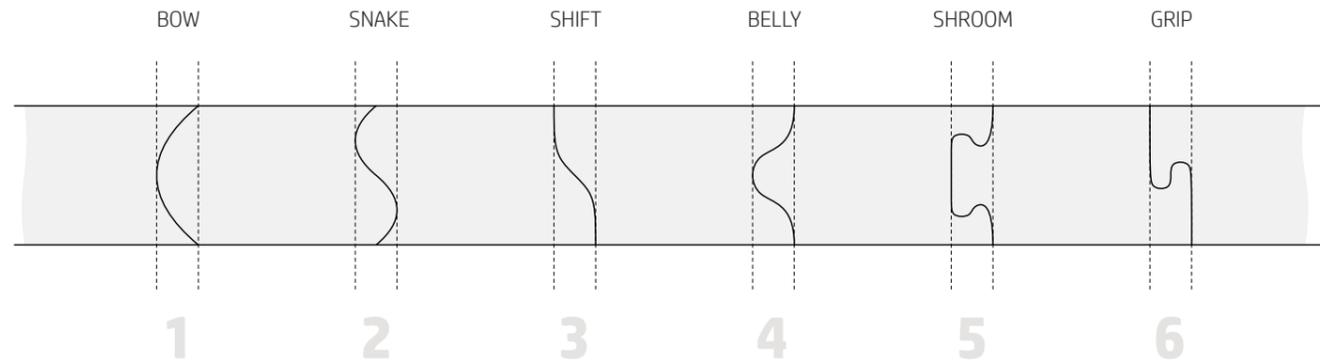
Figure 68: Six different interlocking forms to be investigated.
