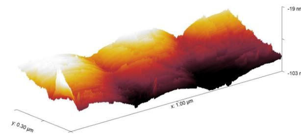
Figure 107: 3D visualisation surface profile of a  $1 \times 0,3 \mu\text{m}$  area with AFM, showing the different roughness in nano scale in which the extreme peaks have a difference of only 84 nm.
