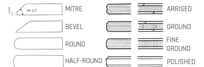
Figure 35: Edge work and beveling [left] and edge types and finishing [right]. Source: (Wurm, 2007)
