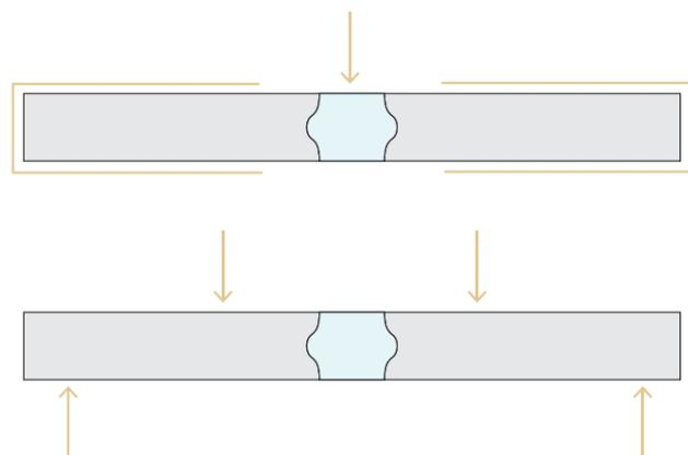
Figure 116: Visualisation of a direct shear test (top) and a 4-point bending test.
