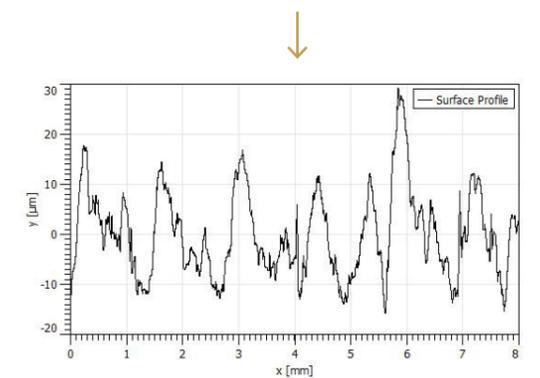
Figure 109: Correct data by leveling for a more accurate average surface roughness calculation after measuring with Dektak.
