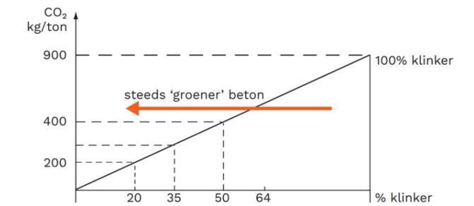
Figure 58: Table showing the less clinkers used in a concrete composition, the lower the carbon emissions thus 'greener' concrete (Betonhuis, 2020).
