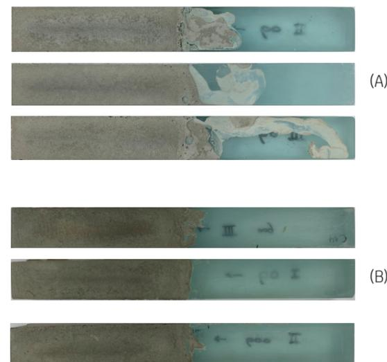
Figure 96: Compacting on the vibrating table causes the concrete to come beneath the glass (A). With a more self-compacting type of concrete, less vibration is necessary, allowing the concrete to stay in place better (B).
