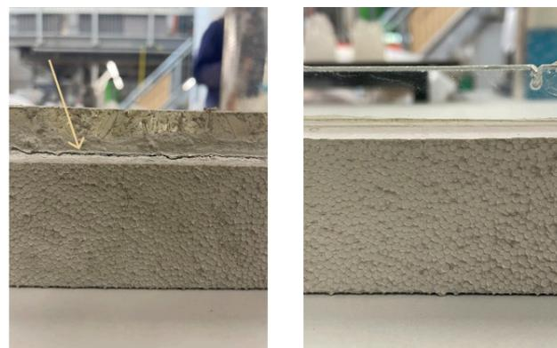
Figure 62: Cracks along the glass edge due to the drying of concrete mixes with lower workability.
