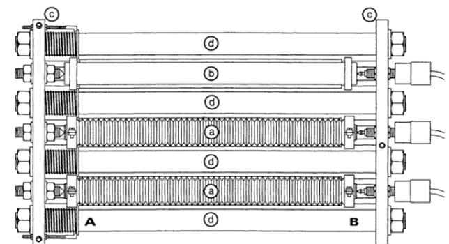
Figure 63: A dilatometer frame with specimens of 300 mm.
