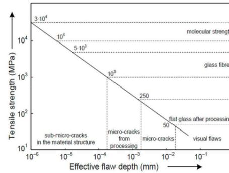
Figure 24: Rough estimated ratio between tensile strength and effective flaw depth. Source (Balkow, 1999)
