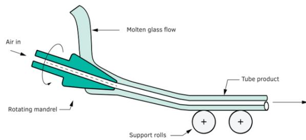
Figure 31: Principle of the danner process. Source: (Oikonomopoulou, 2019)
