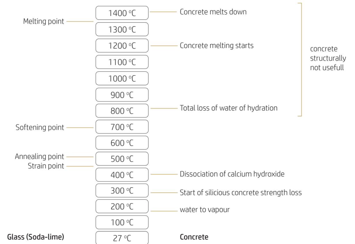
Figure 135: specific temperature properties for glass and concrete, showing the higher melting point of soda-lime glass compared to the thermal degradation point of concrete.
