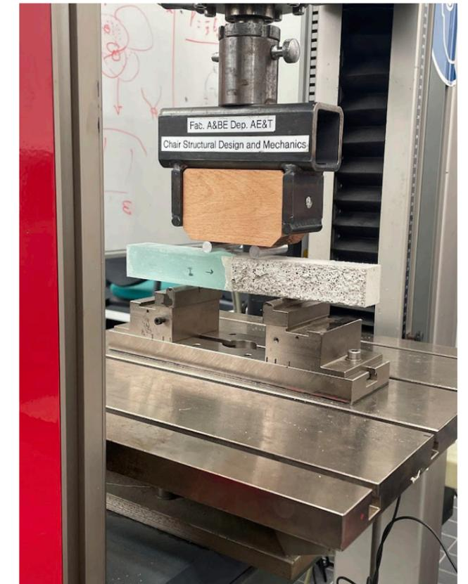
Figure 98: Test set-up of 4-point bending after the second pouring at Materials lab (ME). Testing a concrete-glass interface of a 30x30x240 mm beam with 50/100 support.
