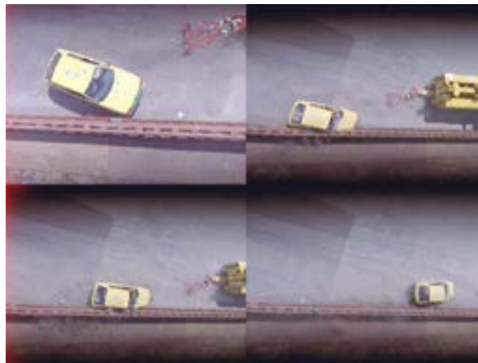
Figure 8. Top view with a high speed camera of the car impact on the guardrail, Full-scale test with a 900 kg car (Test TB 11 according to EN 1317)
