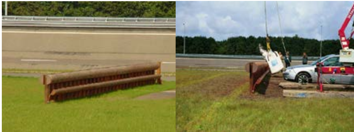
Figure 7. 18-meter prototype of guardrail and sandbag test
