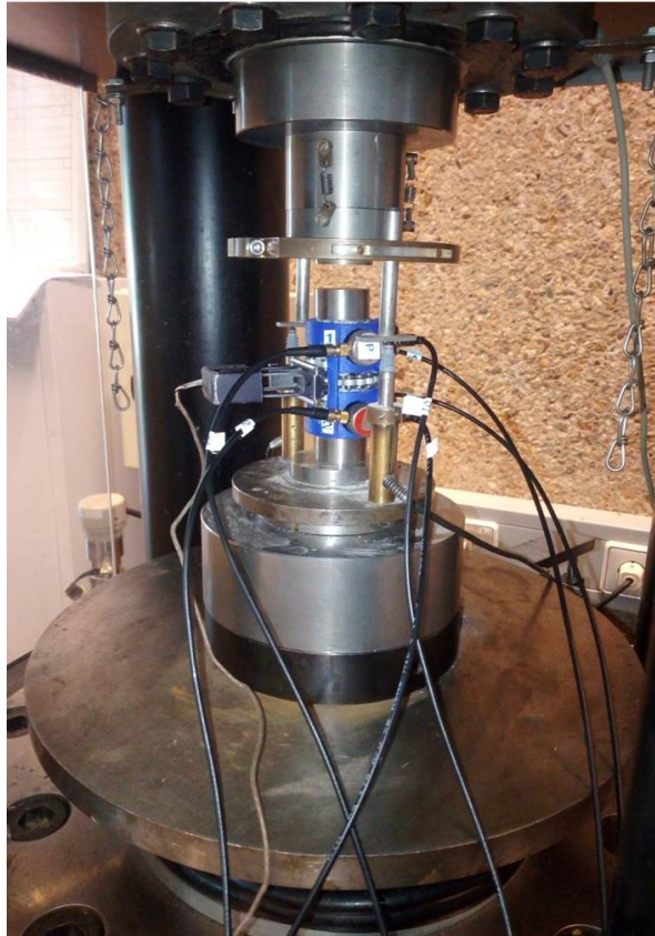
Figure 5.4: Picture of the experimental set up to collect the stress, strain data and the acoustic activity
