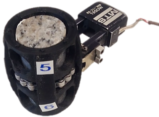
Figure 5.5: Core in the 3D printed sensory jacket
