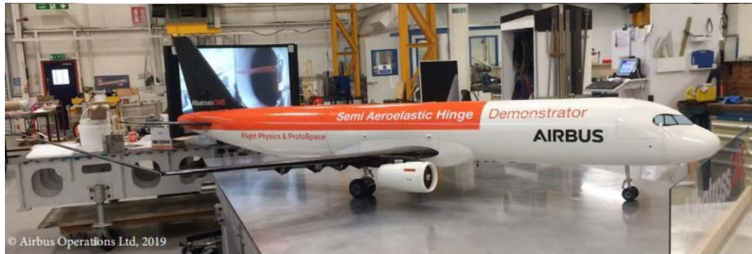
Figure 2.6: The AlbatrossONE scaled flight test demonstrator, taken from [34]
