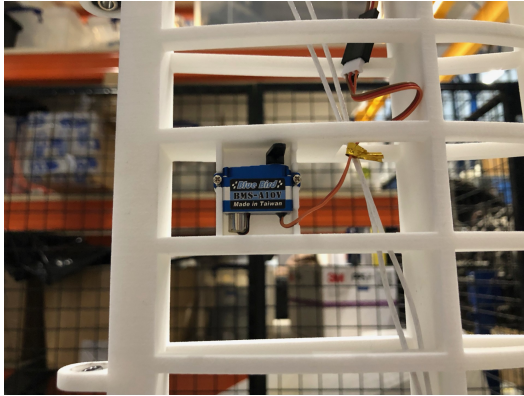
(a) Outboard aileron servo actuator connection without cover
