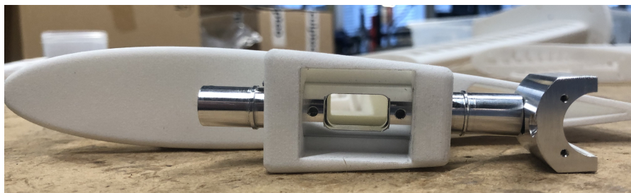
Figure 5.6: Picture of axle, contact plate and wingtip
