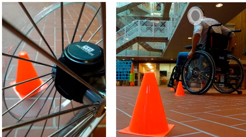
Figure 1. Mounted Movesense sensor and example of the test track.
