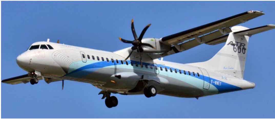
Figure 11.2: Illustration for visual derivation of the type of trailing edge high-lift devices on the ATR 72-600 3
