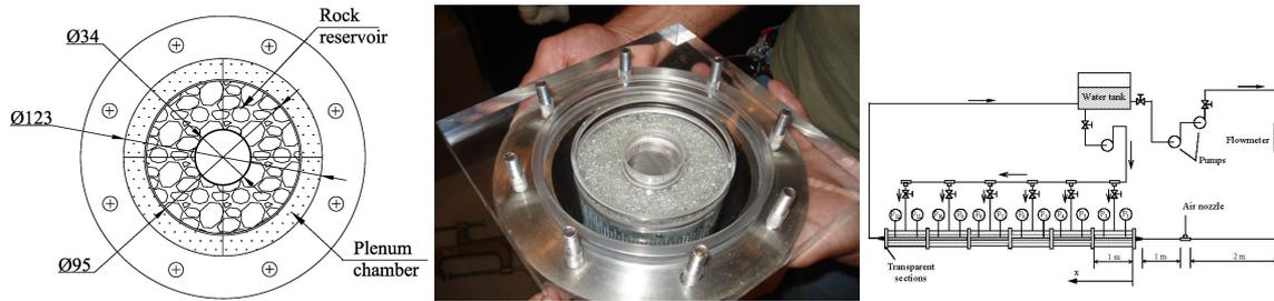
Figure 1: Description of the test section: a) geometric arrangement, b) photograph of actual test section, c) schematic diagram.
