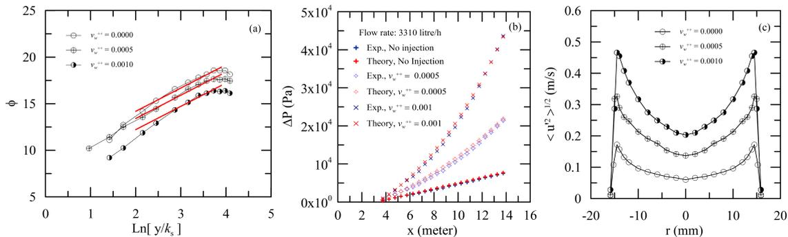
Figure 2: Comparison between the results for unblown case and for the two different transpiration rates studied: a) logarithmic mean velocity distributions, b) pressure drop distributions and c) root mean squared longitudinal fluctuating velocity distributions.
