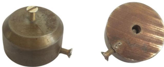
Figure 3.9: Tool used to hold samples during metallographic preparation.
