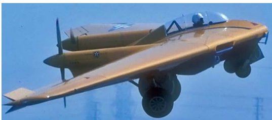
Figure 1.3: The Northrop N-9MB showcasing its clamshell split-flap rudders at the Chino Warbird Show on October 8, 2000 [24]
