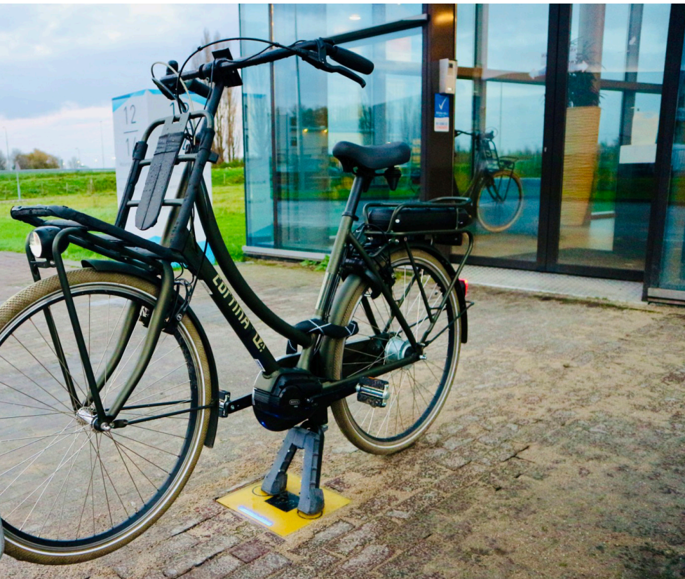
> Figure 34: The first ever installed charging tile in front of the Yes!Delft office at the Molengraaffsingel in Delft
