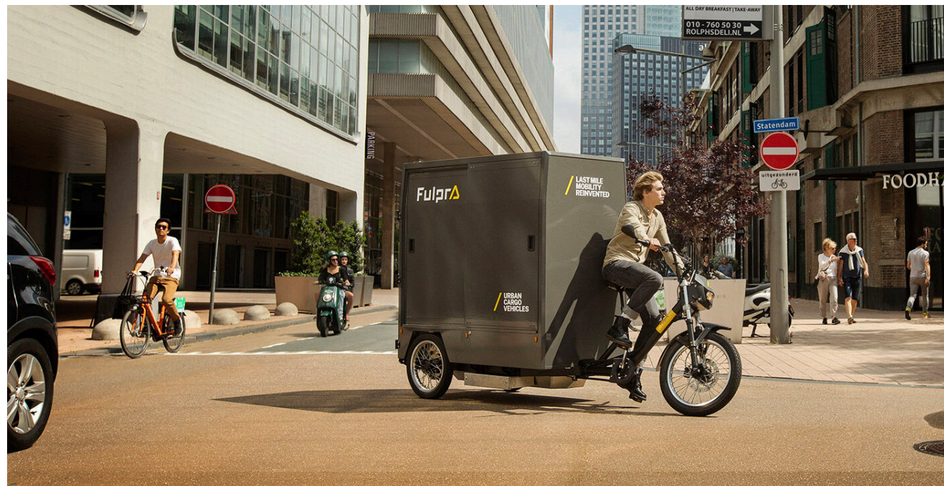
> Figure 17, 18: The parcel-dedicated Fulpra L1 has room for loading two fully loaded trolleys in the back, achieving an unprecedented parcel capacity for cargobikes (image source: Fulpra)
