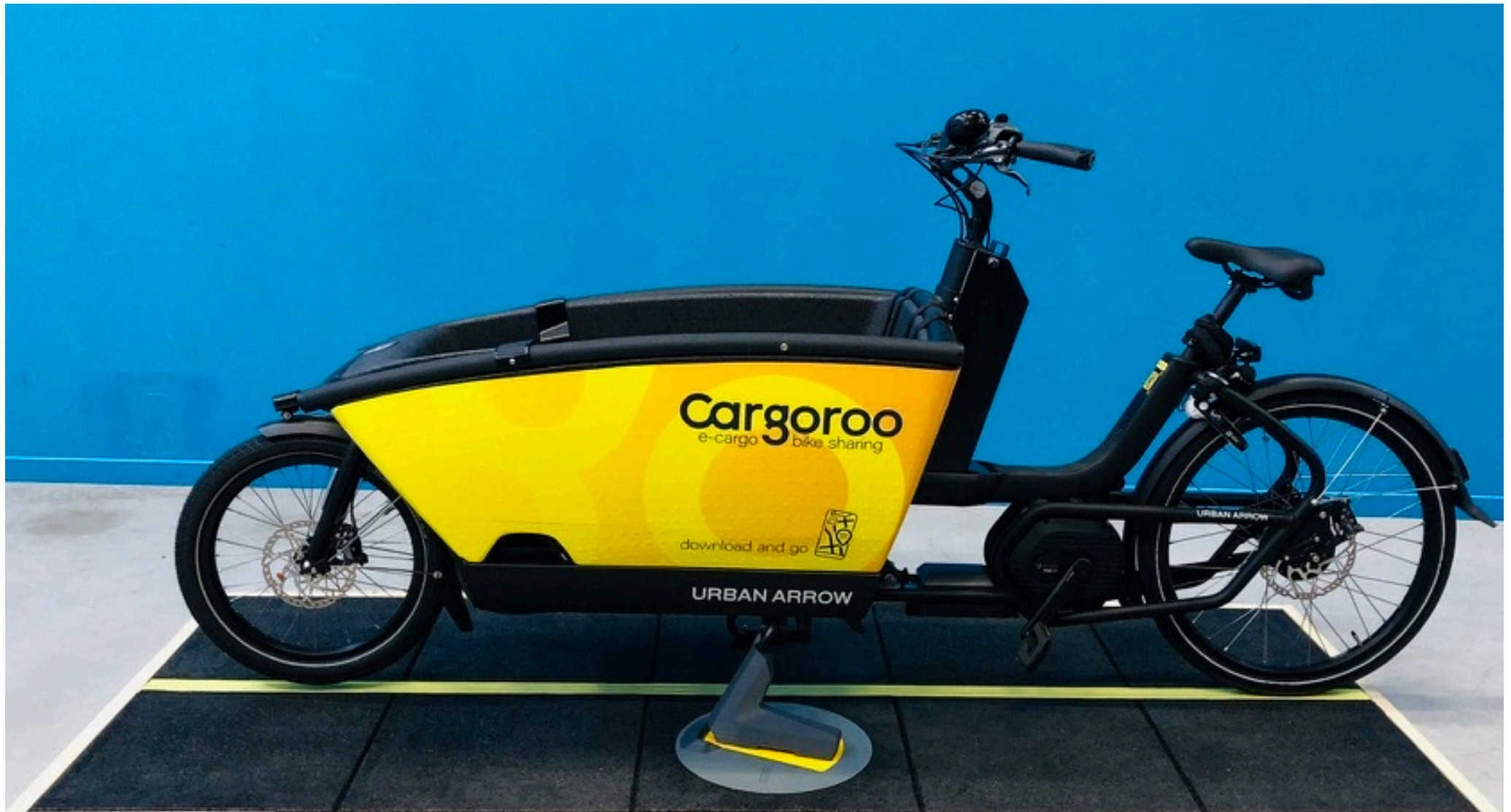
> Figure 60: This physical prototype built for validation purpose illustrates the the placement and dimensions of the charging tile and kickstand relative to the bike
