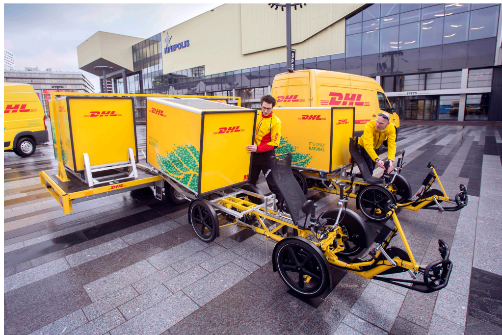
Figure 19: DHL's Cubicycle makes use of preloaded parcel containers to realise a fluent transfer from van to bicycle. The Cubicycle is a branded version of the Velove Armadillo cargobike, designed to revolutionise delivery.
