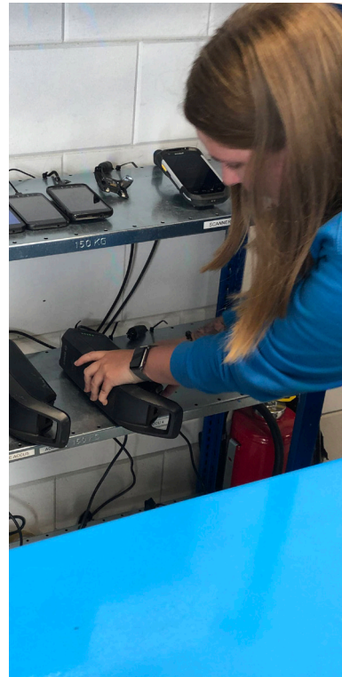
Carry battery to the cabinet and plug it into the charger
