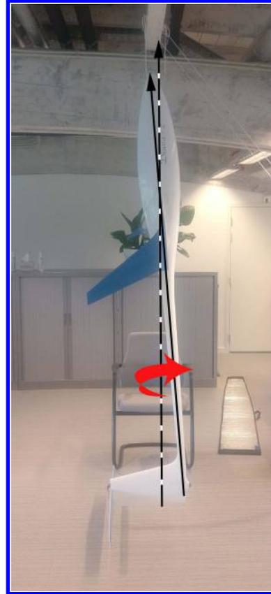
**Fig. 5 Roll moment of inertia setup.**
