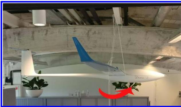
**Fig. 2 Pitch moment of inertia setup.**
