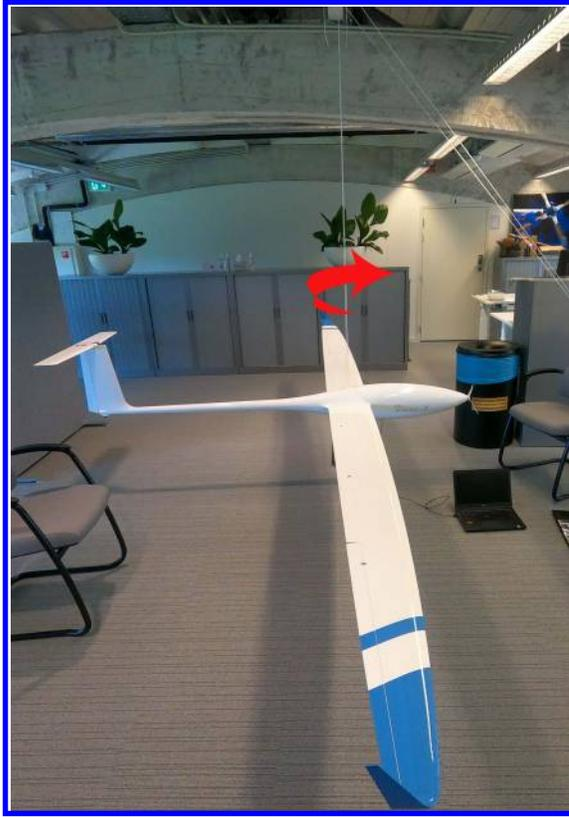
**Fig. 4 Yaw moment of inertia setup.**
