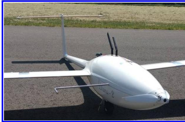
**Fig. 22** Aeroprobe installation location.
