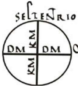
FIG. 2.8 Templum of the earth with Kardo Maximus (KM) and the Decumanus Maximus (DM).
