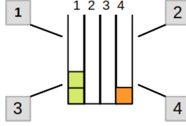
Figure 2.1: Representation of a classical resource sharing station using a Max Weight scheduler (center) with four users (squares).
