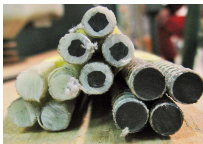
(a) From left to right GFRP, C-GFRP and CFRP reinforcement bars [Prokeš, 2018].
