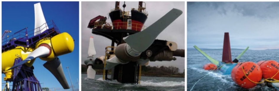
Figure 1.9: Various tidal energy converters with FRP blades [Dawson et al., 2018].
