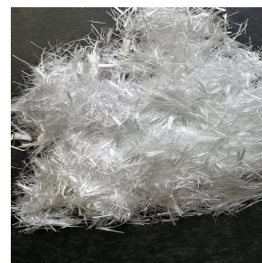
(b) Glass fibres used to construct fibre reinforced concrete [Alibaba, 2019].
