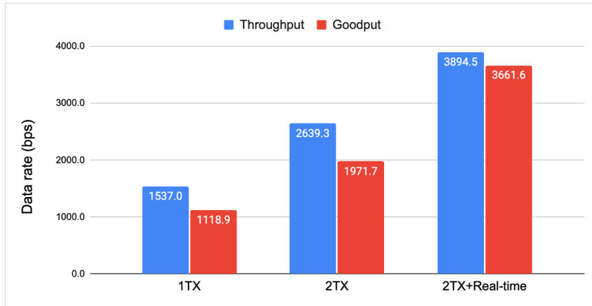
Figure 5.2: Data rate improvements by deploying 2 transmitters and real-time image reading. The First 2 columns indicate data rates with a 15-FPS transmitter and a receiver recording a video at 30 FPS. The 2 columns in the middle indicate data rates with two 15-FPS transmitters and a receiver recording a video at 30 FPS. The last two columns indicate data rates with two 15-FPS transmitters and a receiver reading images at 30 FPS in real time.
