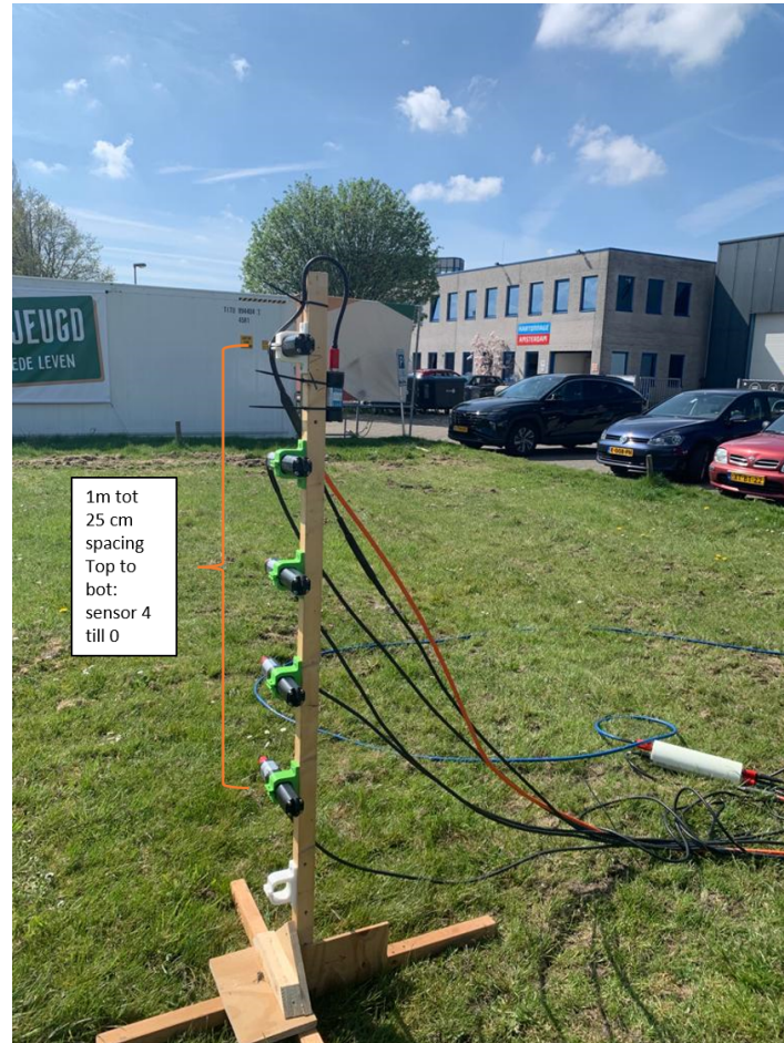
Figure 4-1: The picture of the sensor array shows 5 fluxgate magnetometers in a vertical array, placed in light green holders. The FGM's alignment is measured by an inertial motion unit, or IMU, which is attached to the pole. The sensor setup consists of a pole with sensors spaced 25 cm away from each other. The bottom sensor is located at a height of 0.5m, and the top sensor at 1.5m. The cables run to a white capture unit which pairs the information and sends it to a field laptop.
