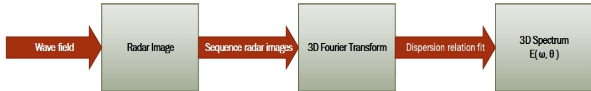
Figure 2.7: Radar image processing schematically illustrated
