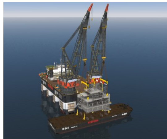
Figure 5.6: Screen-shot of simulation in K-Sim: H-541 Barge and Thialf with Theboud Compression Topside in cranes.
