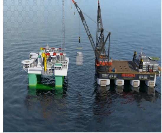
Figure 5.2: Screen-shot of simulation in K-Sim: Gjøa platform and Thialf with Skarfjell module in crane
