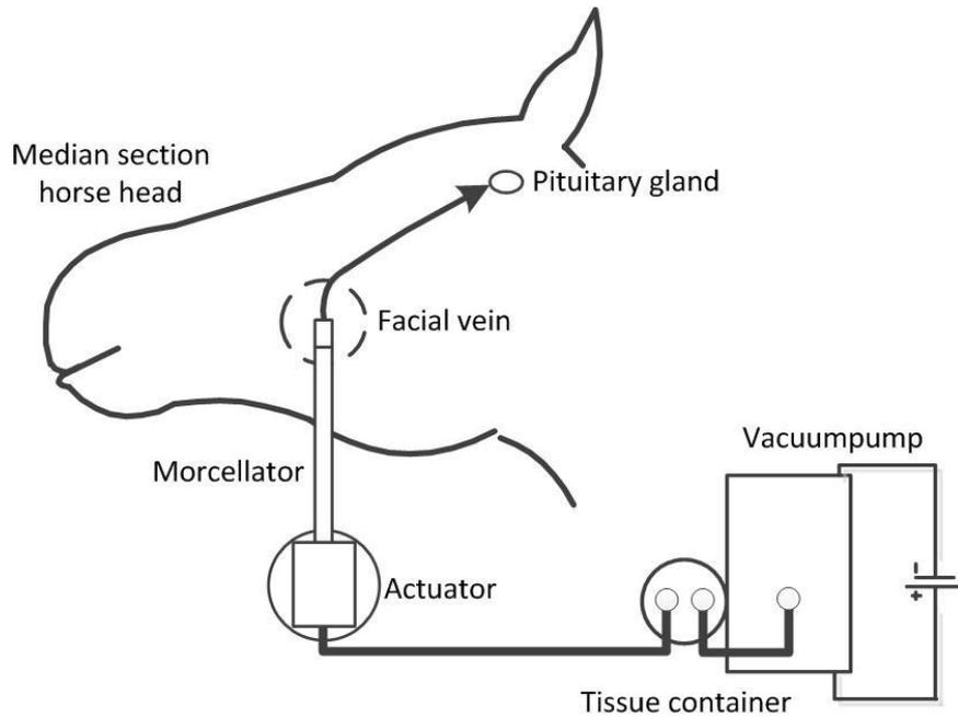
Fig. 47: Test set-up during proof of principle experiment.
