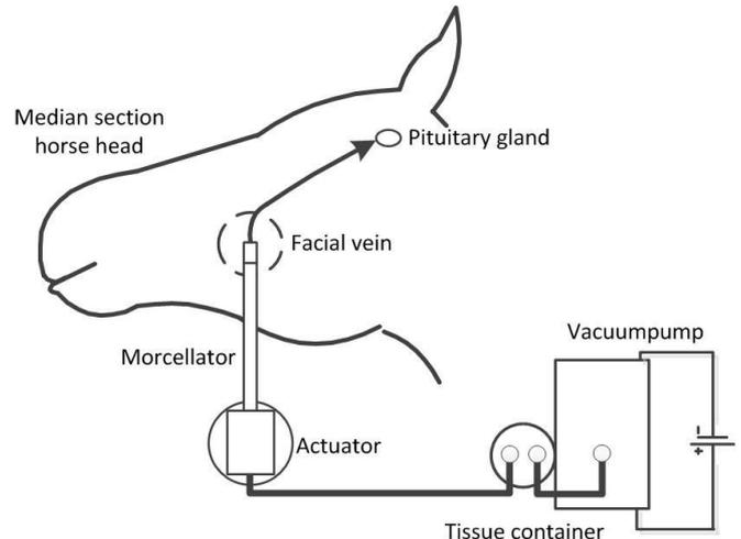
Fig. 23: Schematic illustration of test set-up during experiment.
