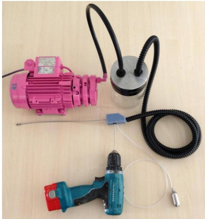
Fig. 22: Total HORSE morcellator assembly including actuator and aspiration system.
