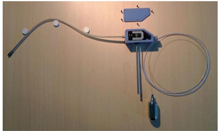
Fig. 16: The HORSE morcellator illustrating the 28 functional parts of the morcellator.
