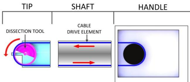
Fig. 12: Final conceptual morcellator design. The red arrows indicate the direction of motion of the resection tool and drive element. The black circle indicates the drive axle of the morcellator.
