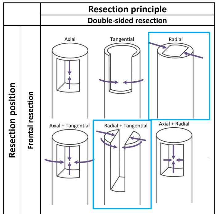
Fig. 11: Section 1:2 from Table 1; frontal double-sided resection. Within this category six potential directions of the resection forces can be utilized for resection; axial, tangential, radial, axial + tangential, radial + tangential and axial + radial resection. Only two feasible directions of resection forces, i.e. radial or radial + tangential resection, comply with the requirements as discussed in this section. These two directions are indicated with the two blue rectangular boxes.
