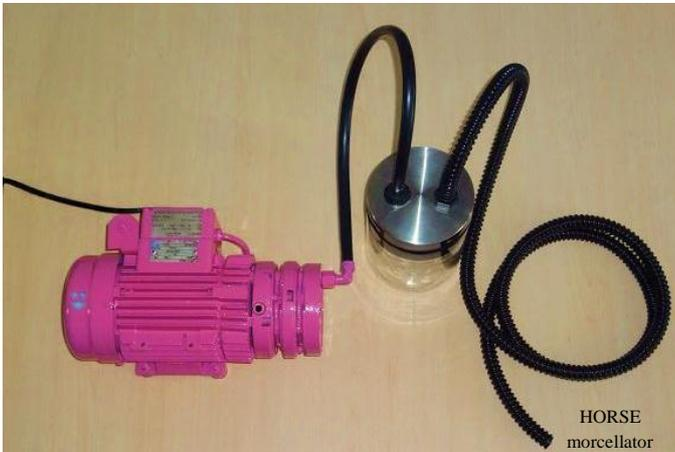
Fig. 20: Aspiration system. From left to right: vacuum pump (pink), connection tube vacuum pump to tissue container, swivel 9 mm, tissue container, swivel 13 mm, and connection tube tissue container to HORSE morcellator.
