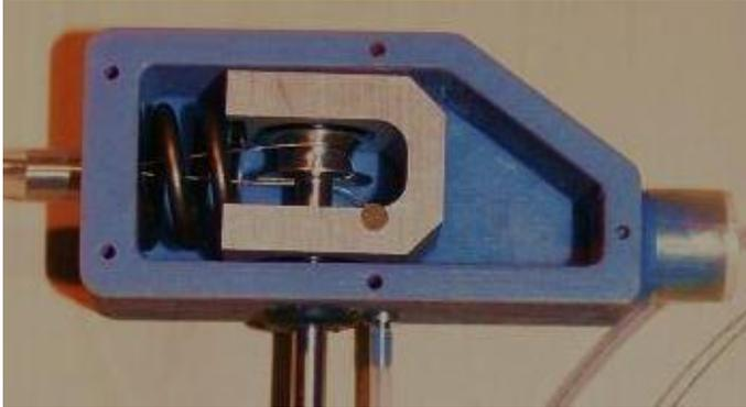
Fig. 19: Handle piece of the HORSE morcellator prototype.
