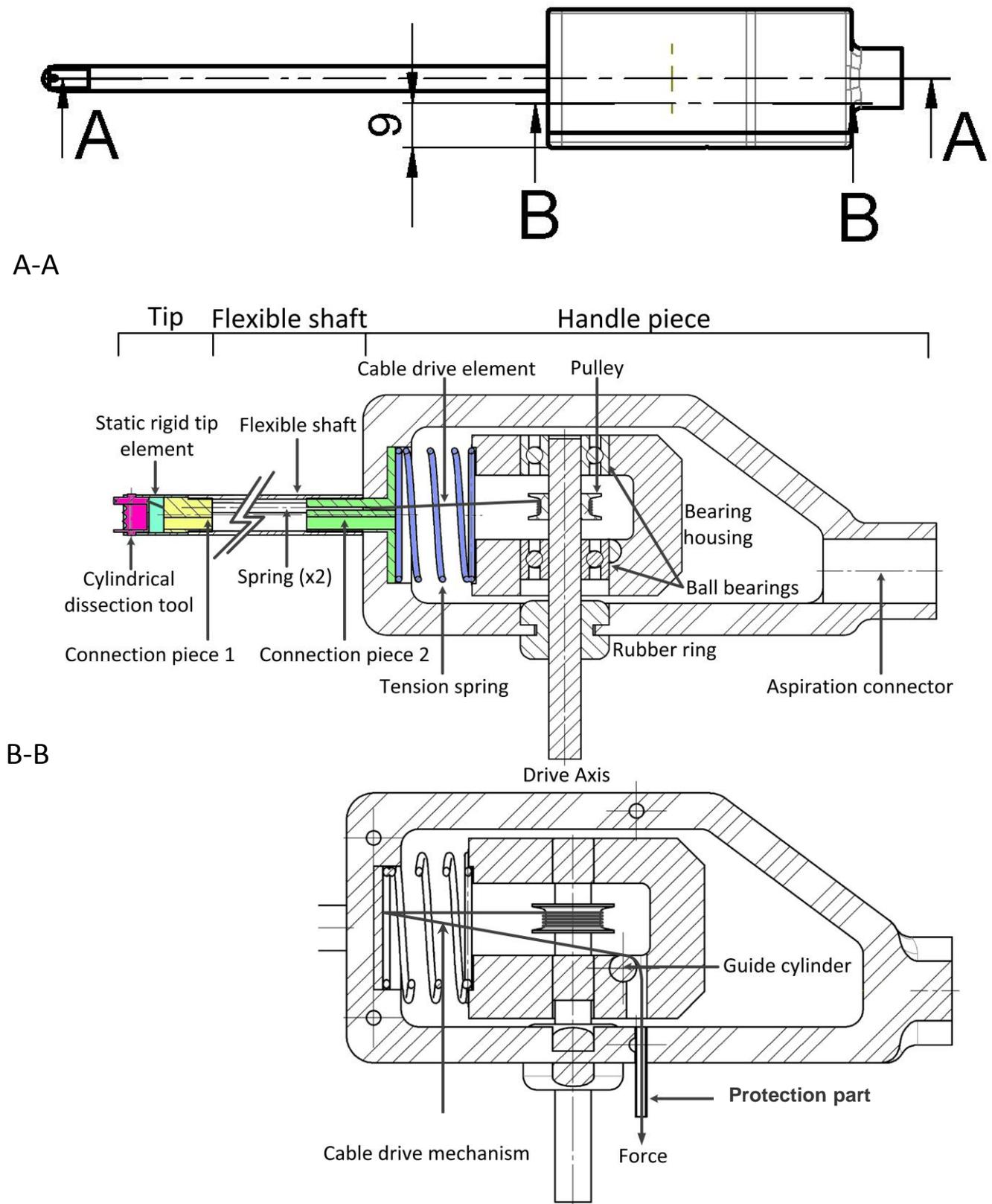
Fig. 15: Schematic representation of the final design. Above: Top view of the HORSE morcellator. Middle: Section A-A representing a median cross-section of the HORSE morcellator. Below: Section B-B representing a cross-section 9 mm from the indicated axis to visualize the cable drive mechanism of the HORSE morcellator.
