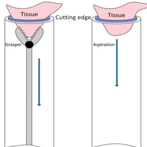
Fig. 4: Morcellation contact initiation and transportation methods. Left: manual approach using a minimal invasive grasper for contact initiation with the cutting edge (purple) and tissue (pink) transportation. Right: aspiration approach using pressure difference for contact initiation with the cutting edge (purple) and tissue (pink) transportation. The blue arrows indicate the direction of the force on the tissue and tissue transportation direction.
