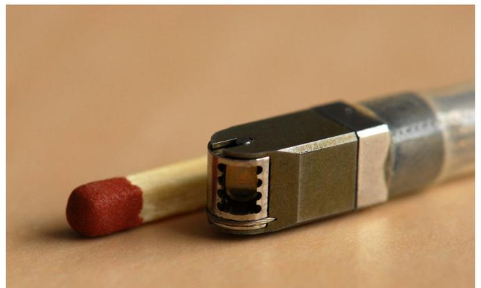
Fig. 18: Assembled tip of the HORSE morcellator prototype.
