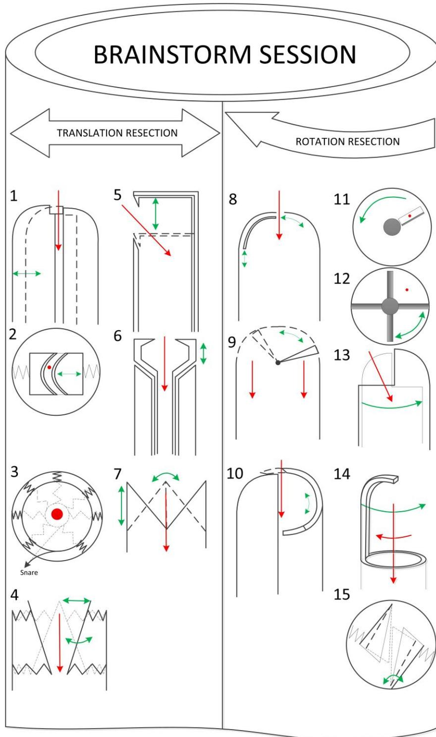
Fig. 45: Brainstorm session 1, design solutions are subdivided into the direction of motion of the resection tool; translation or rotation. The red arrow indicates the direction of the tissue and the green arrows indicate the direction of motion of the resection tool.
