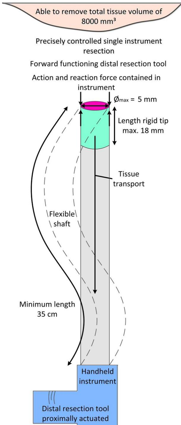
Fig. 13: Graphical representation of the design requirements discussed in the previous sections.
