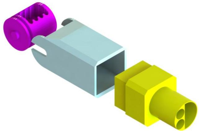
Fig. 14: The tip of the morcellator. From left to right: resection tool, static rigid tip element, and connection piece.
