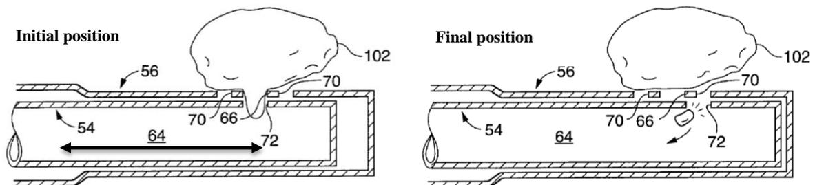
Fig. 38: Coherent EPM shown in patent US 006.156.049 A. The cutting tool of the instrument entails a reciprocating inner tube. The direction of the inner cutting tool is indicated with the arrow. 54: inner tube, 56: outer tube, 64: aspiration channel, 66: aperture outer tube, 70: ports, 72: aperture inner tube, 102: target tissue [38].
