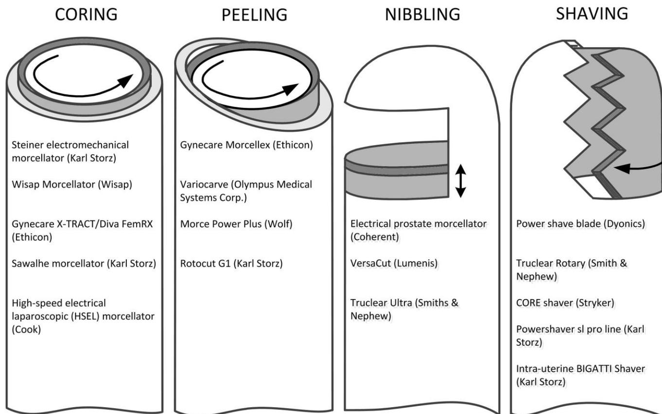
Fig. 5: Schematic illustrations of mechanical morcellator types, i.e. coring, peeling, nibbling and shaving, found in literature with corresponding clinical morcellators currently in use. The resection tool is indicated in grey and the cutting edge of the morcellator in dark grey. The black arrows indicate the direction of motion of the resection tool [21]. For extra information and illustrations of the different morcellator refer to Appendix B.
