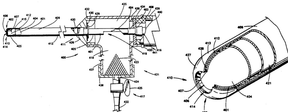
Fig. 34: HSEL Morcellator (Cook). Left: handpiece HSEL morcellator, Right: tip of the HSEL morcellator. Most relevant indicated numbers: 402: distal end of the morcellator, 406: distal opening of the inner rotary cutting member tube, 407: rotary open ended cutting edge, 414: distal opening of the outer tube [33].
