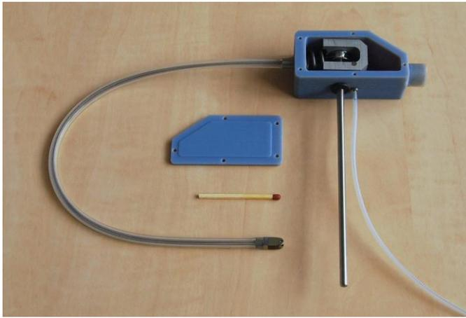
Fig. 21: Assembled HORSE morcellator prototype.
