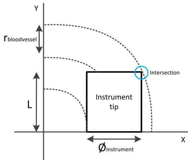
Fig. 10: Schematic overview of a blood vessel (indicated with the dotted line) with an inserted catheter with a rigid tip.
