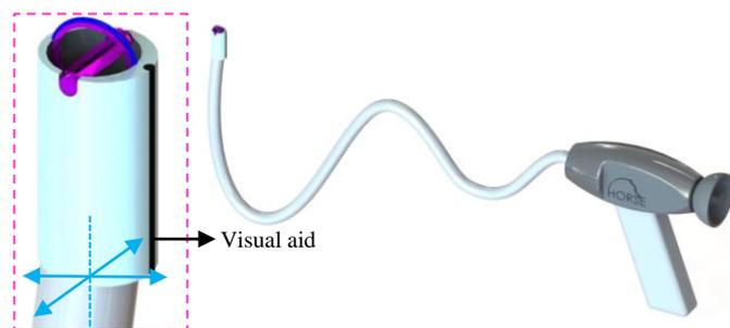
Fig. 27: Future vision of the HORSE morcellator after redesign. The blue arrows indicate the active steerable degrees of freedom of the tip of the morcellator. The integration of the optical fiber or other visual aid in the tip of the morcellator is indicated in black. The resection tool is indicated in pink, the cable drive element in blue and the rigid tip of the morcellator in light green.
