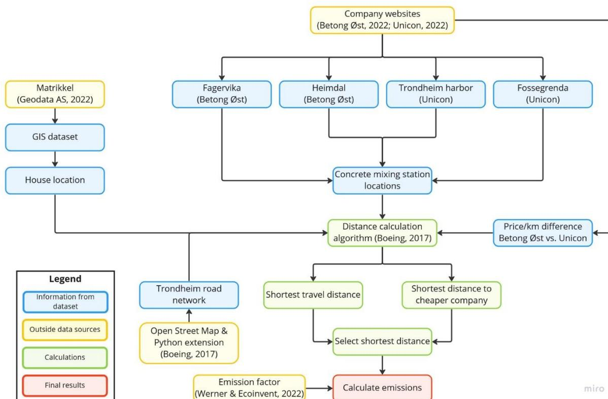
Figure 4.2-4: Data flow overview of the transport distance model.
