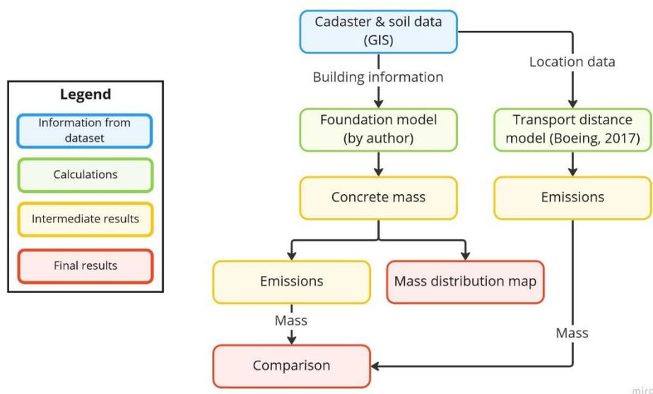
Figure 3.5-1: Overview of how the different approaches interact with each other. Cadaster data from Geodata AS (2022) and soil data from NGU (2022).
