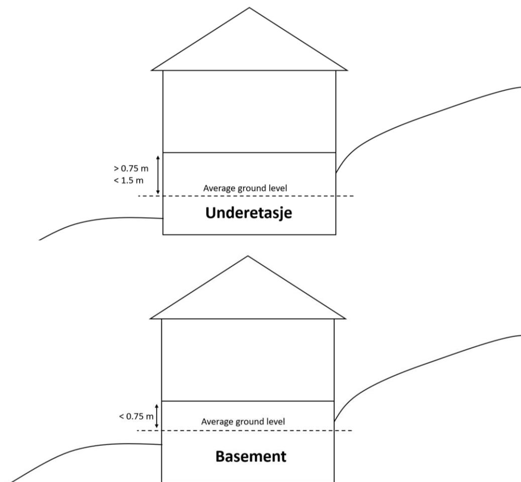
Figure 4.2-1: Visualization of an "underetasje" and a basement, showing their similarity. Underetasjer are simply a basement that comes higher out of the ground (Kartverket, 2023).
