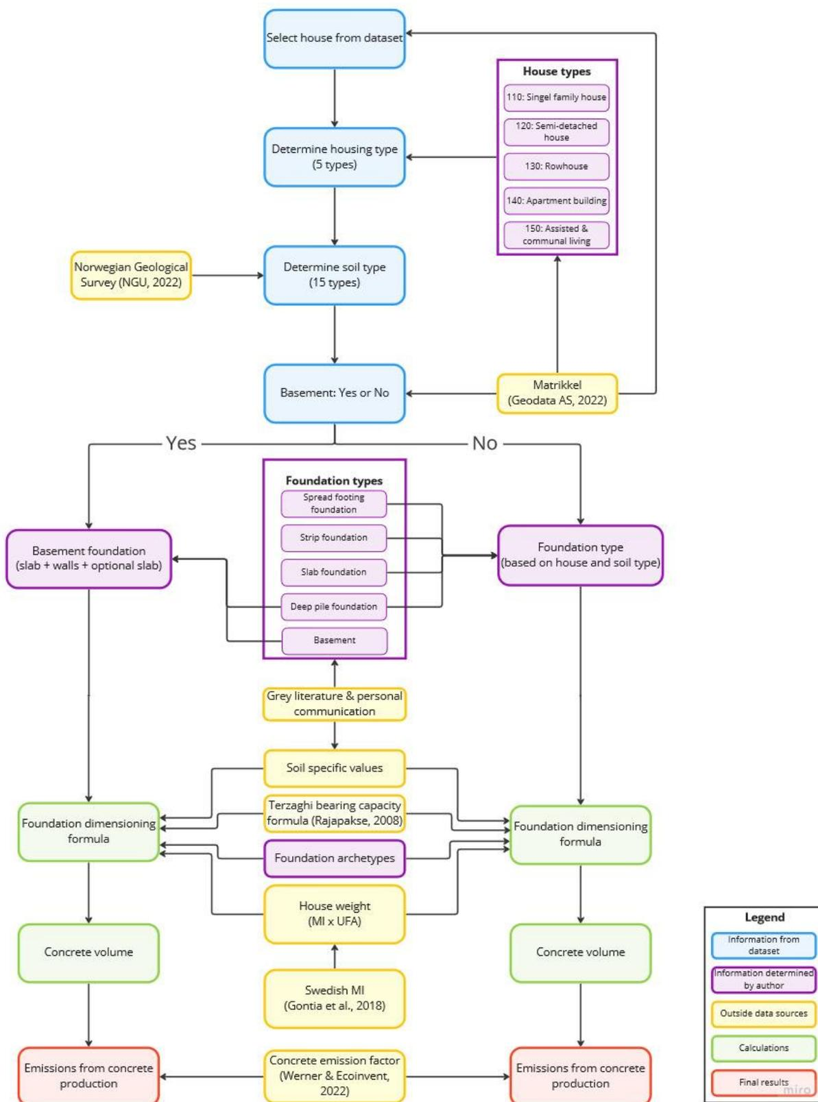
Figure 4.2-3: Foundation model data flow.
