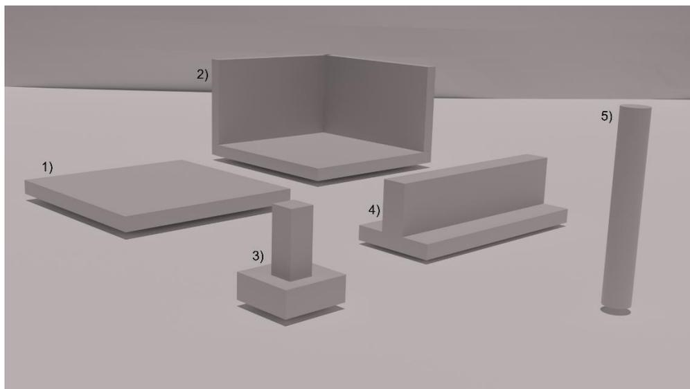
Figure 4.2-2: Visualization of the five foundation types. From left to right is 1) slab, 2) basement, 3) spread footing, 4) strip, 5) deep pile foundation (image made by the author).
