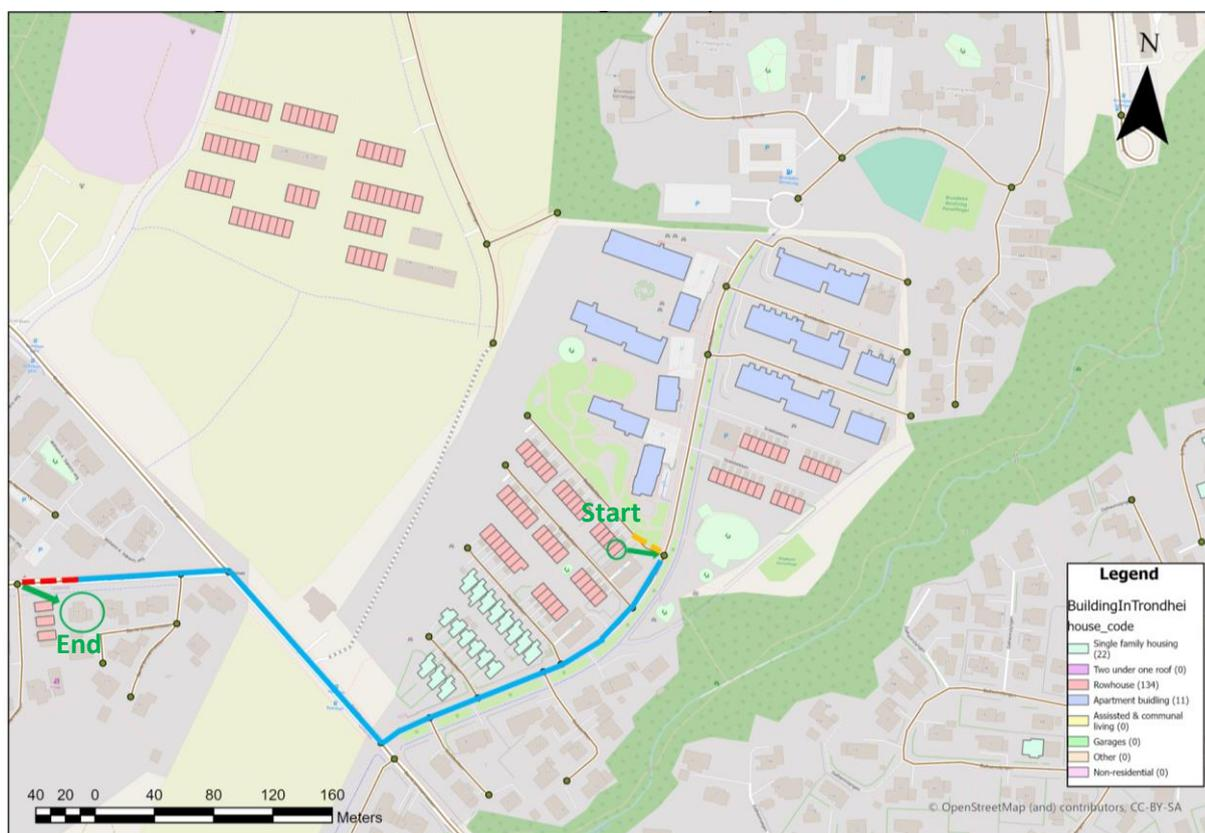
Figure 4.2-5: Visualization of inaccuracies of path calculations. The blue + red path is calculated as total distance. However, the orange line at the start should be added, while the red line at the end should be disregarded. This is due to the node guided algorithm. For more on this check the OSMnx documentation [online](#).
