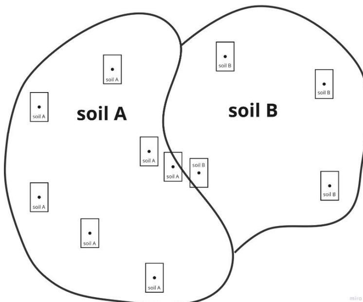
Figure 4.1-1: Visualization of the spatial join function in ArcGIS Pro based on a shape's midpoint.
