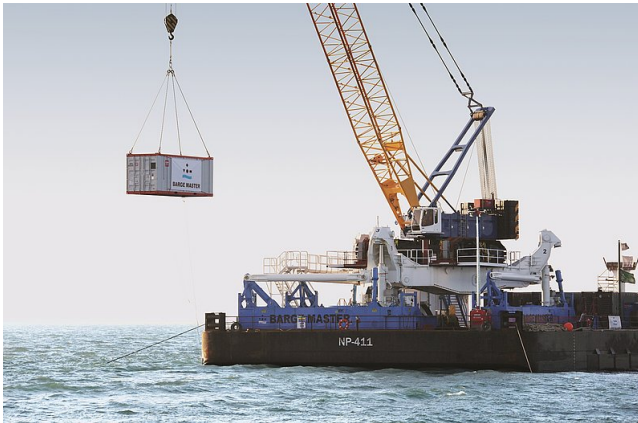
Figure 2.6: Direct ship motion compensation (Barge Master, 2020).
