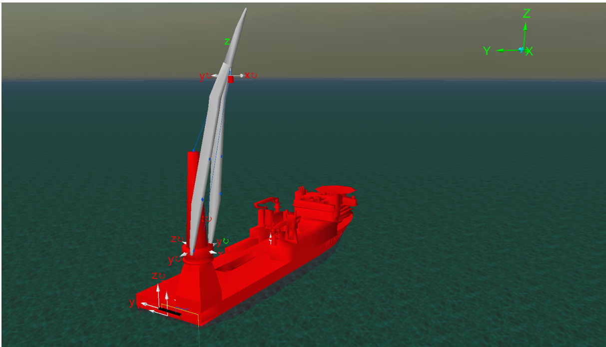
Figure 5.1: HLV Aegir including earth-fixed heave compensation modelled in OrcaFlex.
