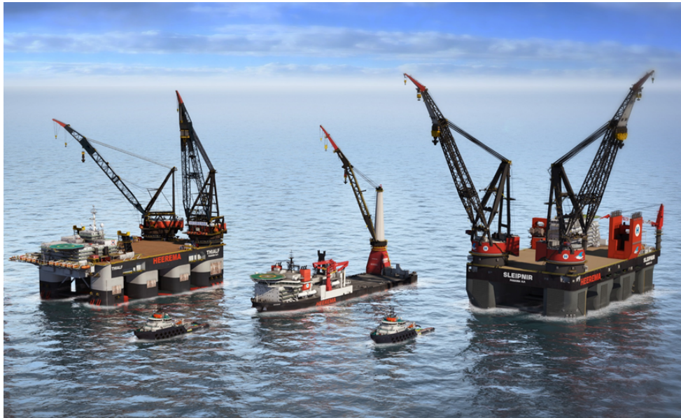
Figure 1.2: Part of Heerema's fleet. From left to right, top to bottom: SSCV Thialf, HLV Aegir, SSCV Sleipnir, Kolga (tug), Bylgia (tug). Source: Heerema
