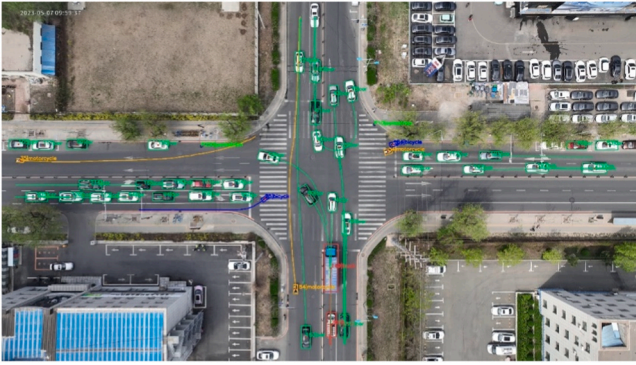
Fig. 1. A sample of Signalized Intersection Dataset (SIND) [58]. (Green label refers to the car class, light green label refers to the pedestrian class, yellow label refers to the motorcycle class, green label refers to the bicycle class, red label refers to the specific object used in [58]).
