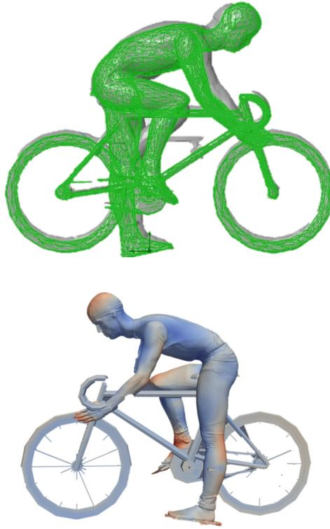
**Fig. 4.** (a) Visualizing the differences in side view overlapped. The green mesh is rigged, the grey is true. (b) Difference in surfaces highlighted by the intensity of the blue and red colors, mapped on to the surface of the rigged scan
