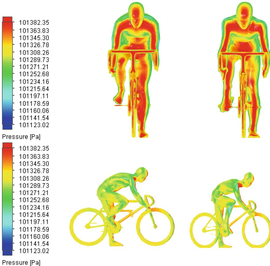
**Fig. 5.** Pressure maps in the front view (top) and side view (bottom). The force per unit area for each cell is calculated and color-coded based on the numeric value. The net pressure of all these cells (in the direction of wind) is the drag force. This figure illustrates that majority of the pressure from the air occurs in the front, the first surface that encounters oncoming air. The maps also confirm minute differences in the two shapes (see neck and left leg).
