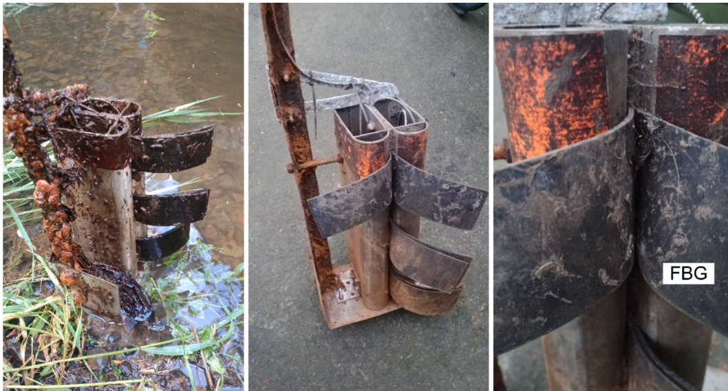
Fig. 13. Images showing the recovered VFS including the delaminated fins and exposed FBG. Top fin deliberately splayed open to show FBG.
