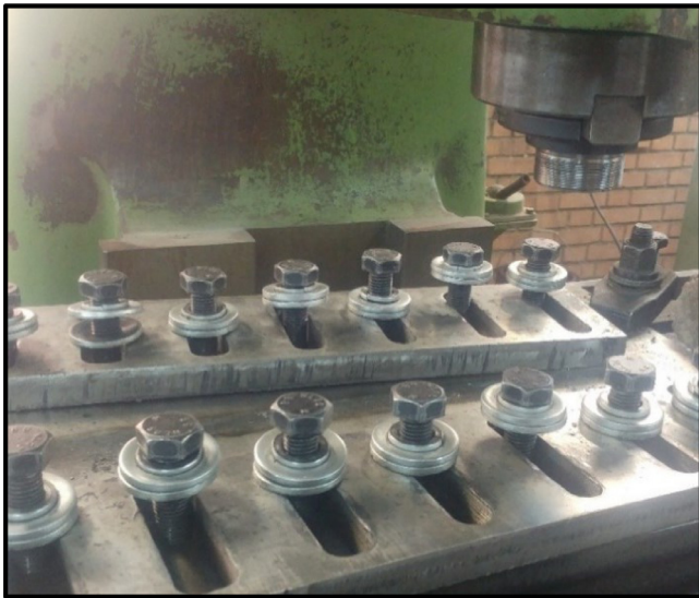
Fig. 3. FSW machinery equipment with side clamping facility.
